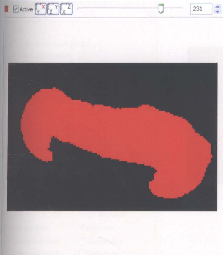
Figure 117 Apply cavity fill in Simpleware
