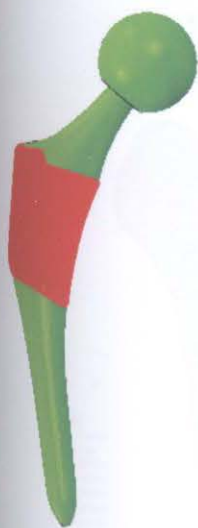
Figure 133 Friction Zone (Red) Frictionless Zone (Green)
