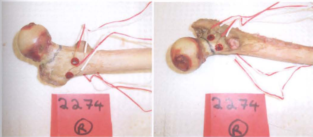
Figure 92 Representative strain gauge attachment to femur
