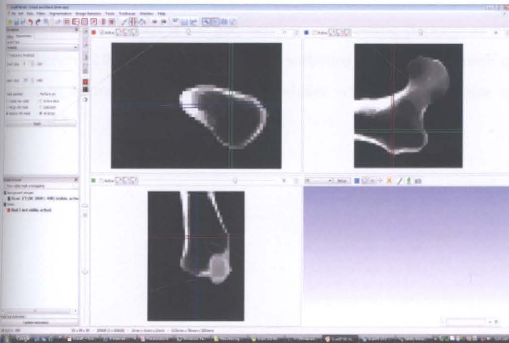
Figure 166 Proximal geometry of femur from CT scan viewed in Simpleware
