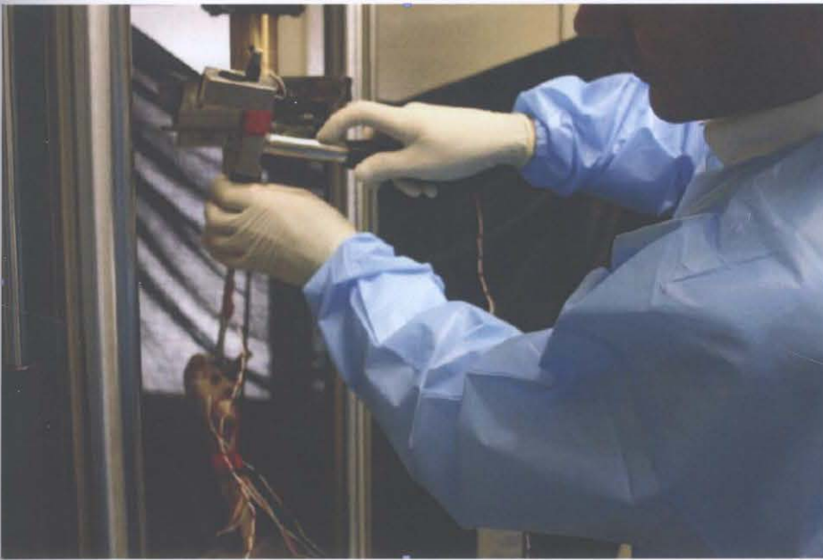
Figure 97 Impaction of stem into femur during testing
