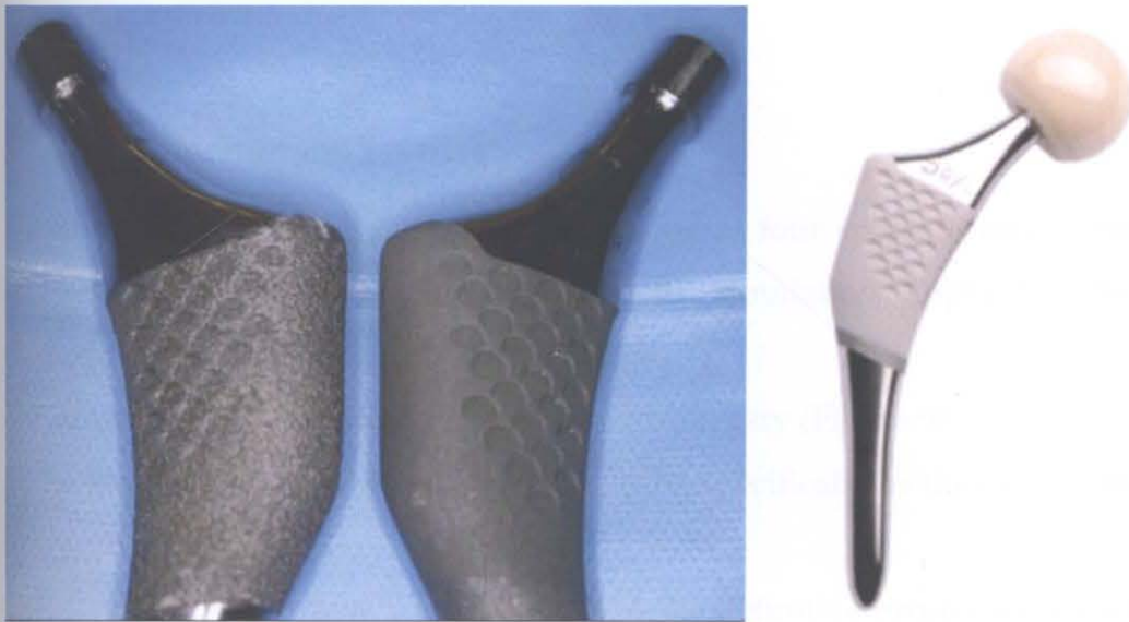
Figure 95 Experimental stems; ABGII Plasma (far left) ABGII NMS (middle left) ABGII Standard (right)
