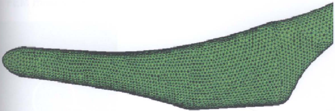
Figure 129 Meshing implant in ABAQUS CAE gives consistent mesh boundary at the interface
