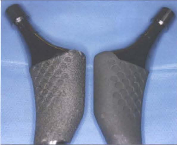
Figure 15 Porous coating only (left) vs HA coating only (implant samples used for testing in chapter 3)
