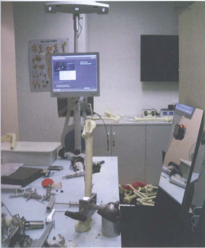
Figure 154 Setup used to record hammer velocity with the Stryker Navigation research version of software
