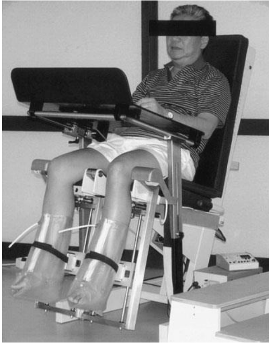
Figure 1. Experimental setup for the assessment of knee joint proprioception, showing the measurement chair control mechanism, handheld button, air splints, and footrest (the moving component of the apparatus).
