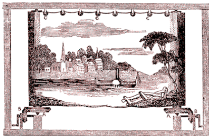
Fig. 4. Illustration of a moving panorama apparatus, John Banvard, 1848. The long strip of painted canvas was mechanically unrolled with the help of a crank handle.
