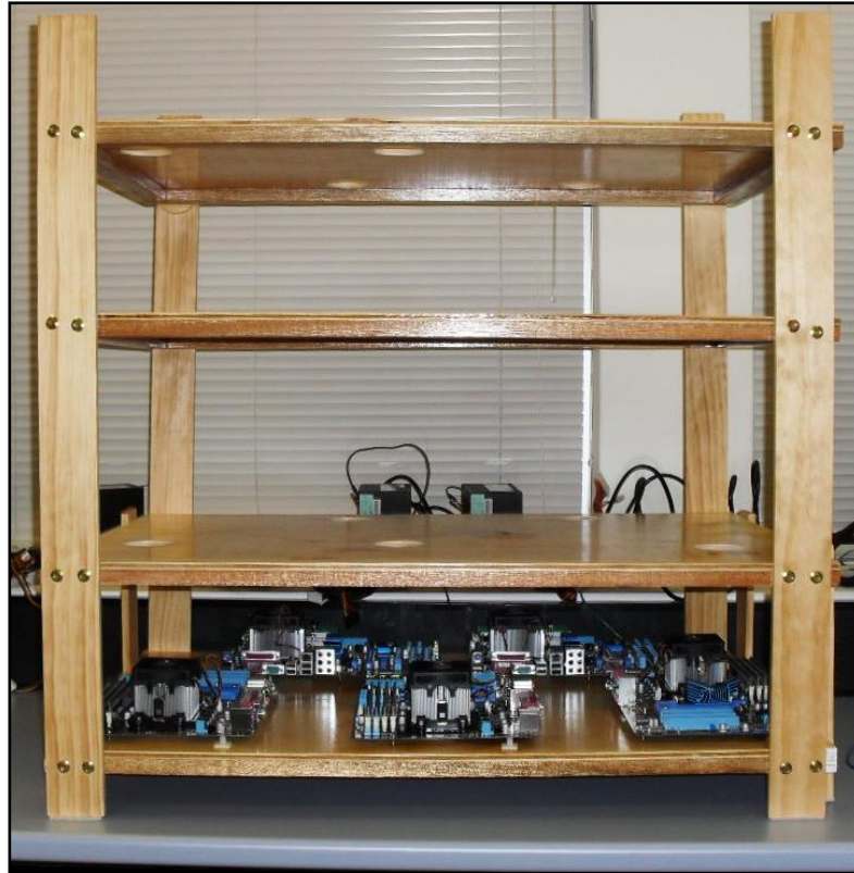
Figure 3.11. Wooden supporting structure for the cluster, with first five motherboards installed on lower level. Holes allowing cables to pass through to adjacent levels may be seen on the second and fourth levels.
