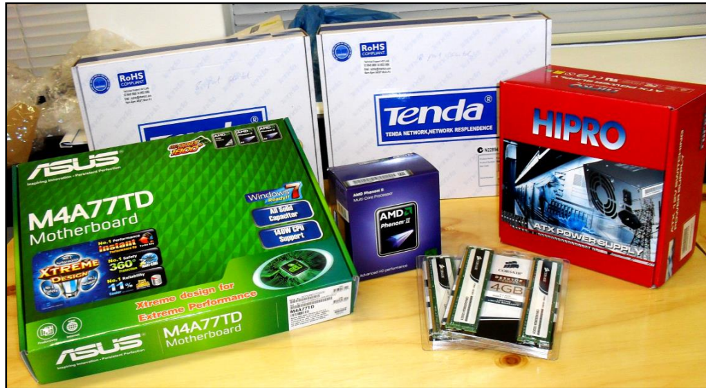
Figure 3.10. Principal hardware components of one node of the high performance cluster, including: a motherboard, CPU, memory modules, power supply unit. The network switch that allowed communication between the nodes is also shown at the rear.
