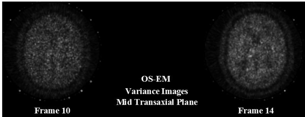
Figure 4.21. Variance images for OS-EM reconstruction, one transaxial slice. Each image is scaled to own maximum.
