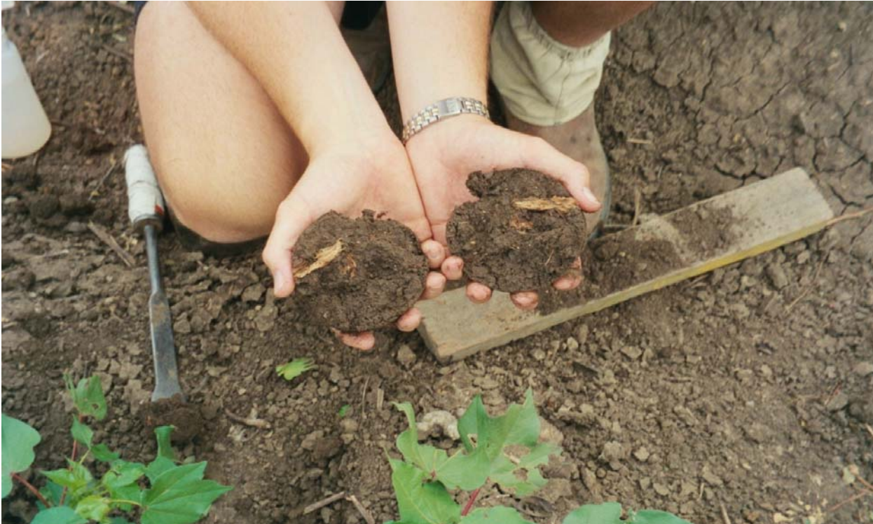
Fig 2.3. Photo illustrating the core break method after a core sample has been broken in half.
