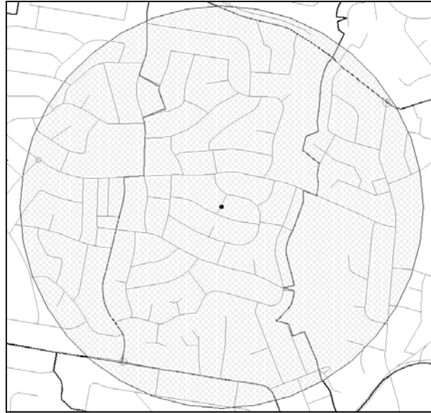
Figure 8.3 A Built Environment with more Pseudo Nodes as a Baseline (Number of Pseudo nodes: 3,240; Source: developed from Sydney GIS layers)
