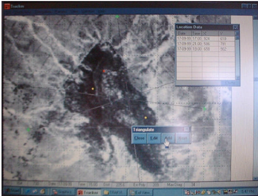
Figure 6.9 Photo reproduction of computer screen showing Tracker 1.0 triangulating compass bearings into XY map coordinates at Site 2. Yellow and red dots indicate animal locations and green crosses tracking stations. Direct image importation was not possible due to software incompatibility while the program is in operation.
