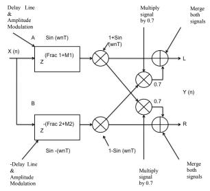
Figure 1.Simulation of rotating speakers [1]
