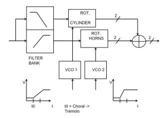
Figure 3. Rotary Speaker Simulation [1]
