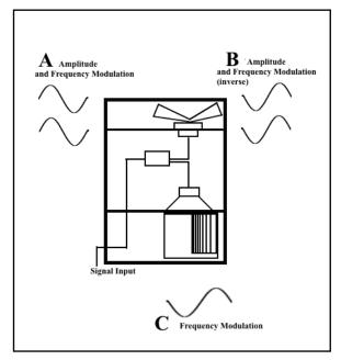
Figure 2. The three main signal components of the rotary loudspeaker effect.
