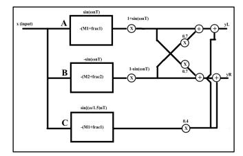
Figure 3. Signal flow diagram of the complete rotary loudspeaker algorithm, beginning with a detail of frequency modulation and finally the processing of the stereo signals.
