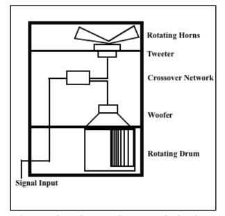
Figure 1. The analogue two-driver rotary loudspeaker to be simulated with ad DSP algorithm.
