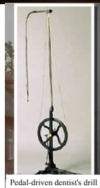
Pedal-driven dentist's drill
