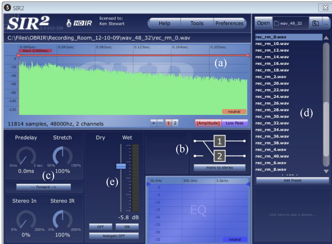
Figure A.11: The SIR2 convolver loaded with an OBRIR in the ‘deg_blks~’ subpatcher in Max/MSP
