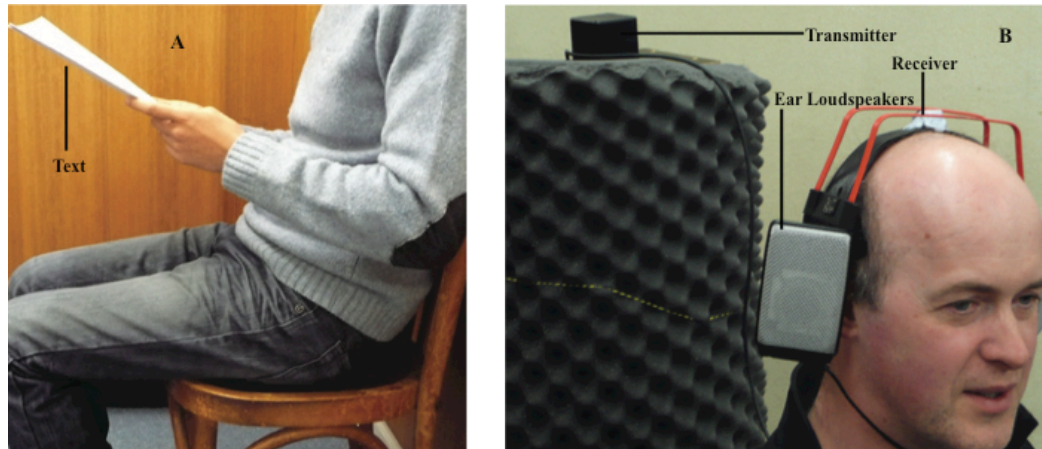
Figure 3.3: The set-up for the readings showing the text being held at a comfortable level (A) and the head-tracking receiver on the ear loudspeakers and the transmitter (B) behind a seated user (not a participant).
