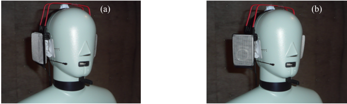
Figure 4.5 (a) The close-to-ear and (b) the maximum angle away-from-ear configurations possible with the AKG K1000 ear-loudspeakers. Here (b) is the preferred position for the current system.
