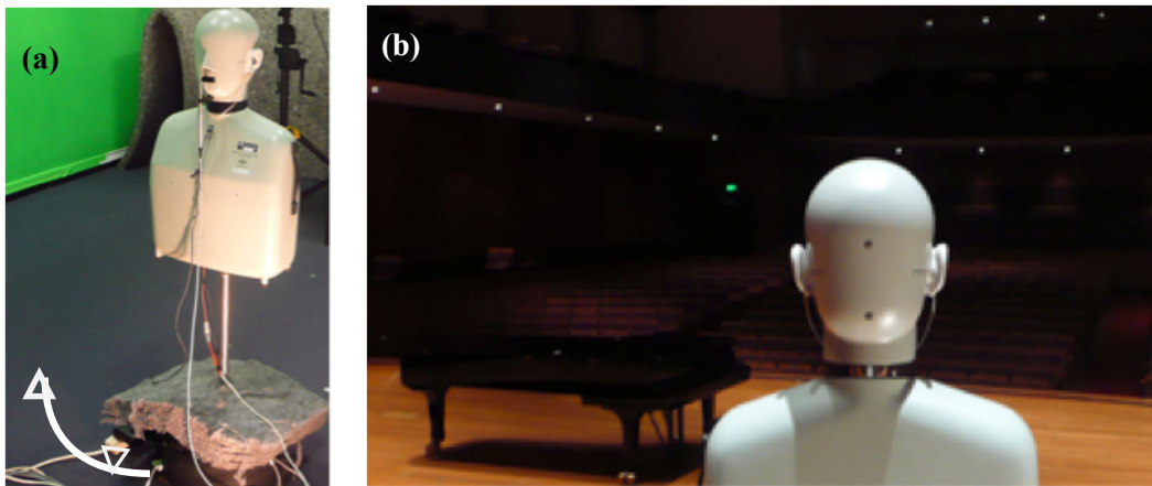
Figure 2.4: (a) The figure shows the HATS mounted on a turntable that can rotate in 2^\circ (can be variable) increments to binaurally scan a room. Also seen are the mouth and ear microphones. (b) The view from behind the HATS in a large room.
