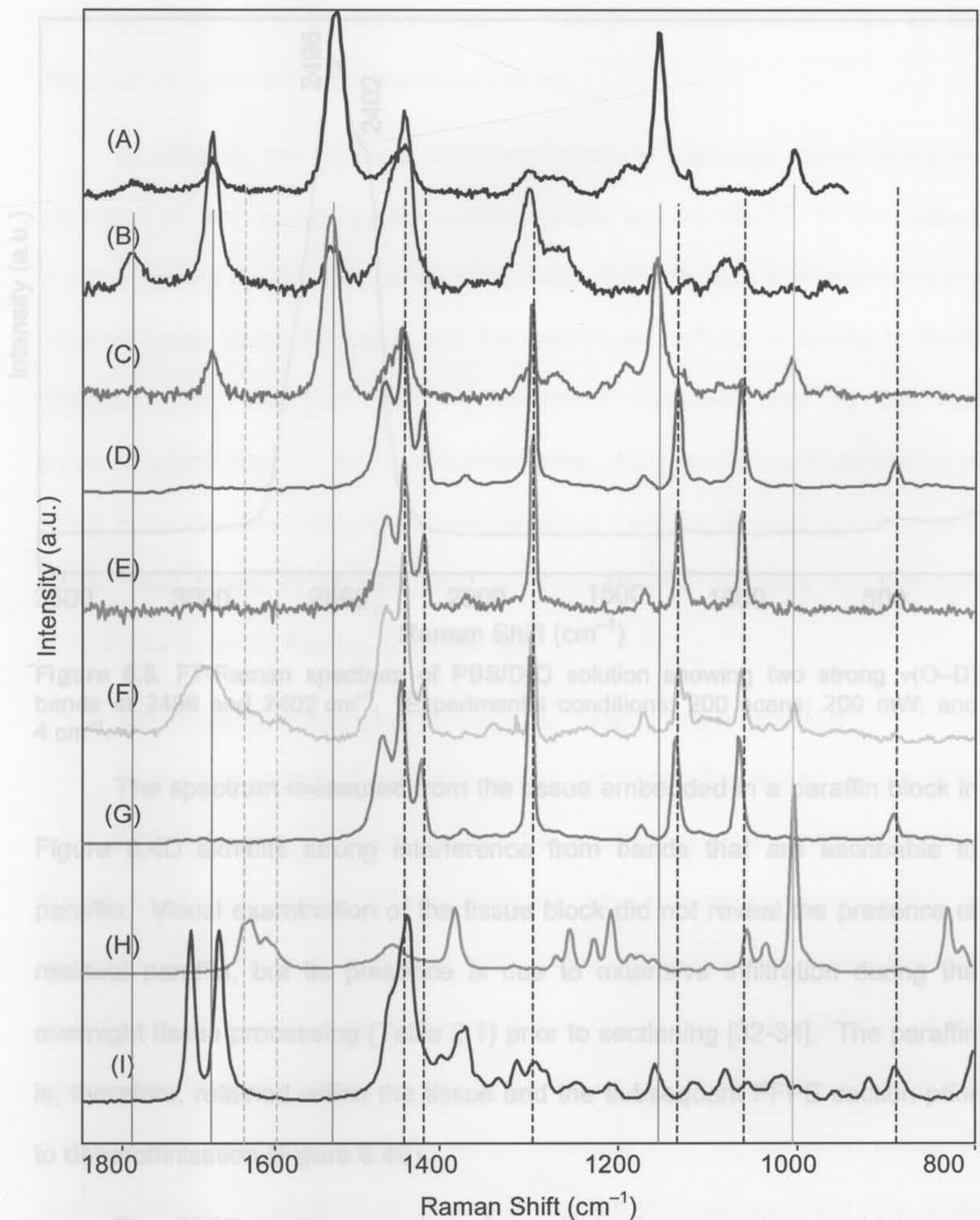
Figure 6.4. Spectral evaluation of a pre-identified (histopathology) IDC lesions as a function of sample processing: (A) “bulk” tissue in PBS/D 2 O; (B) cryosection containing adipose tissue; (C) cryosection without adipose tissue; (D) FFPE tissue block; (E) FFPE section; and (F) deparaffinised FFPE section. Raman spectra of chemical solutions (pathology grades) used in preparation of the FFPE sections: (G) paraffin wax; (H) xylene; and (I) histopure. Experimental conditions: (A–G) \lambda = 514\text{-nm} , \sim 2\text{ mW} at sample, exposure time between 10–60 s with 3 accumulations. (H and I) \lambda = 1064\text{-nm} ; 200 scans; and 4\text{ cm}^{-1} . Bands: blue line: biological components; green line: \beta -carotene; grey dotted line: paraffin; and orange dotted line: deparaffinising agents. Spectra are baseline corrected and are offset for clarity.
