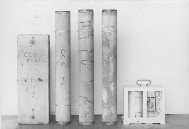
PLATE XXX 8 IN. x 7 IN. AND 4 IN. DIA. SHRINKAGE SPECIMENS, 4 IN. DIA. MODEL COLUMNS
