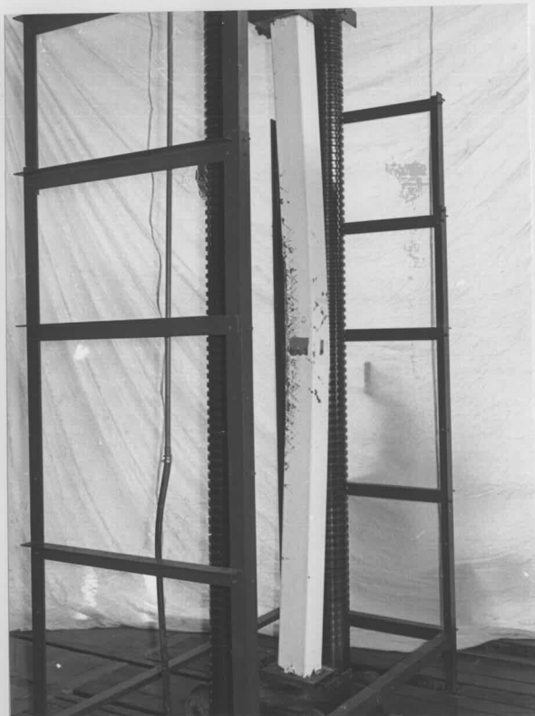
PLATE XXVI YIELDED REGIONS AND DEFORMED SHAPE FOR 6IN. SQUARE COLUMN SHC-8 ( e = 2.5\text{IN.} , \beta = 0^\circ )
