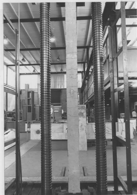
(b) Cracking on South Face
