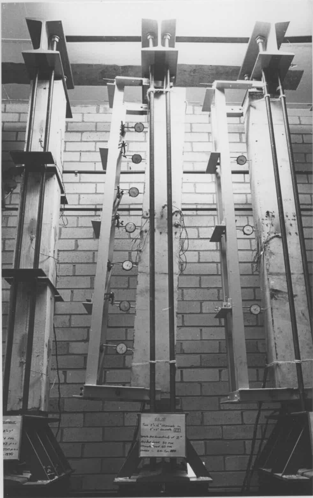
PLATE XLII COLUMNS CC9, CC10 AND CREEP SPECIMENS UNDER SUSTAINED LOAD IN CREEP RIGS
