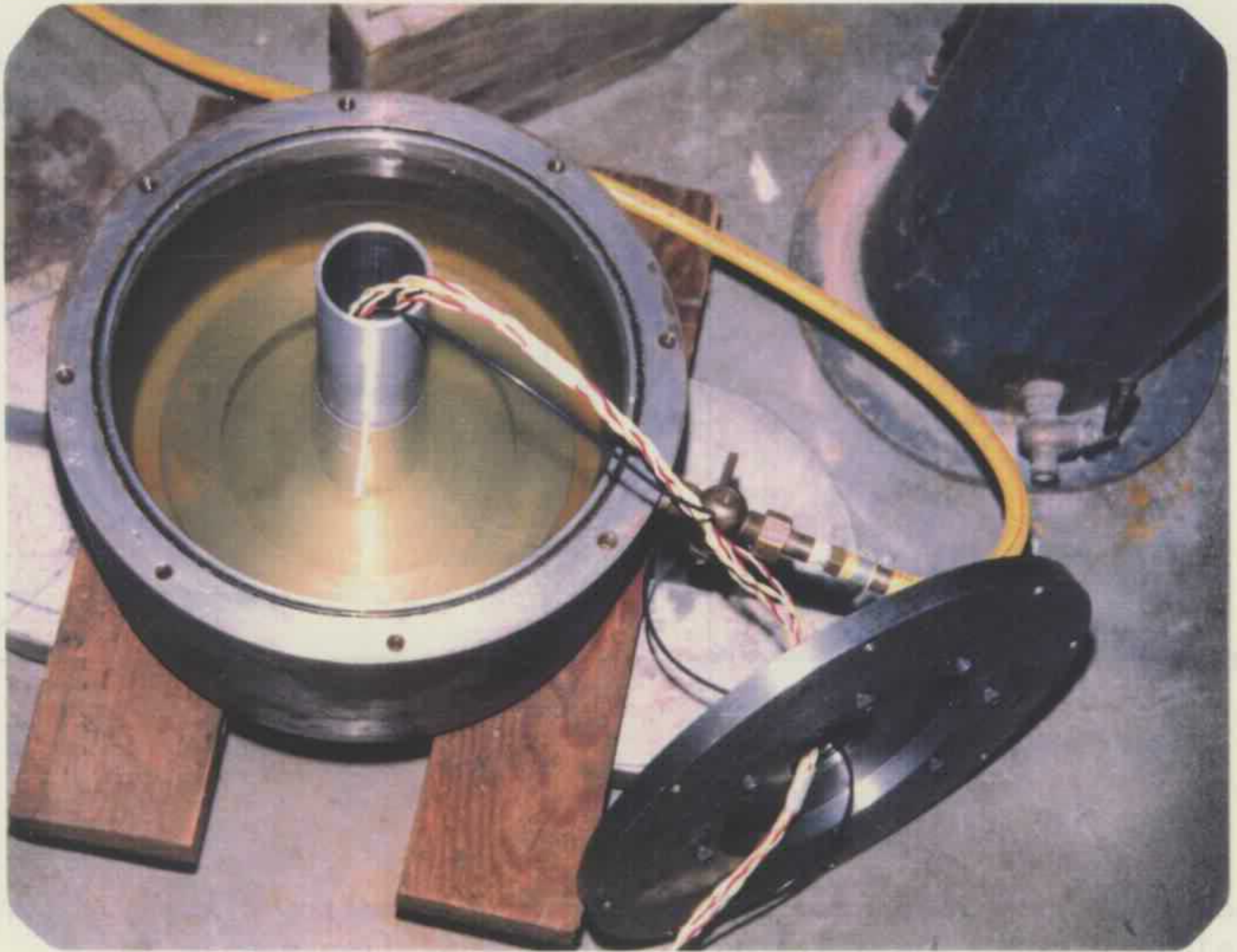
Plate 7.1 Normal stress calibration of instrumented segment (50mm diameter)
