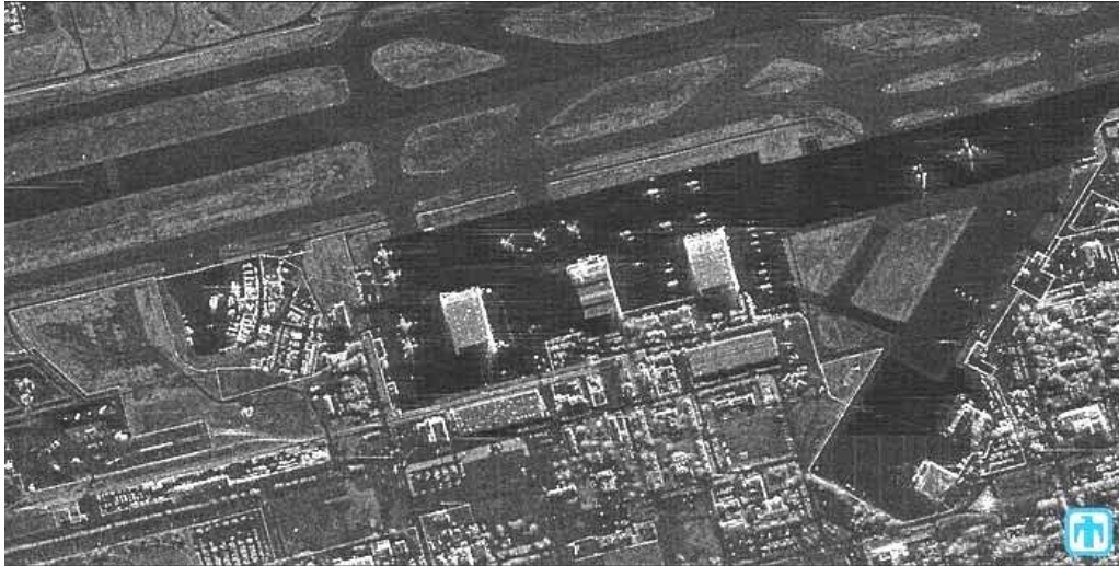
Figure 1.2: Airborne SAR image showing hangars around the Kirtland AFB, Albuquerque, New Mexico, (1m resolution) [10]
