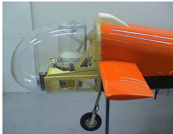
Figure 7.5: Miniature 77GHz radar and mirror scanner mounted on gimbals in the nose of the Brumby Mk-II
