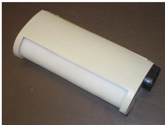
Figure 7.2: Spinning-grating antenna used to achieve a fast azimuth scan rate for range-gate limited radar images
