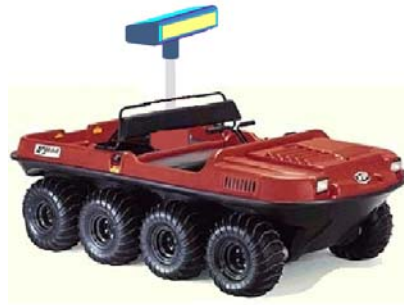
Figure 6.24: Conceptual drawing of an imaging radar mounted on the Argo AGV
