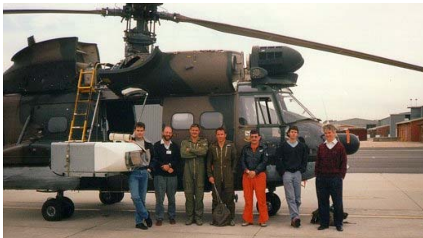
Figure 6.2: Photograph of the radar installed in a pod cantilevered from the side of the Puma helicopter, and the development team, the pilots and engineer
