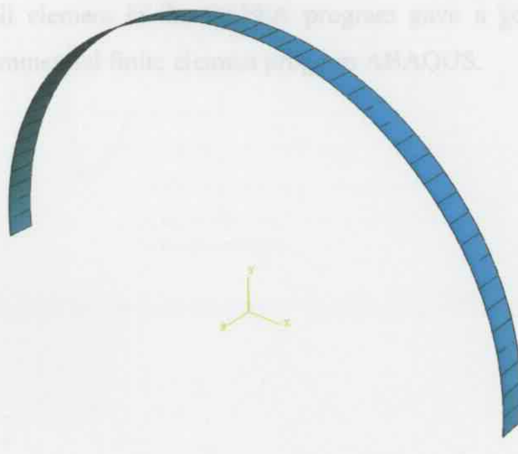
Figure 5.9a: Mesh division of the arch.
