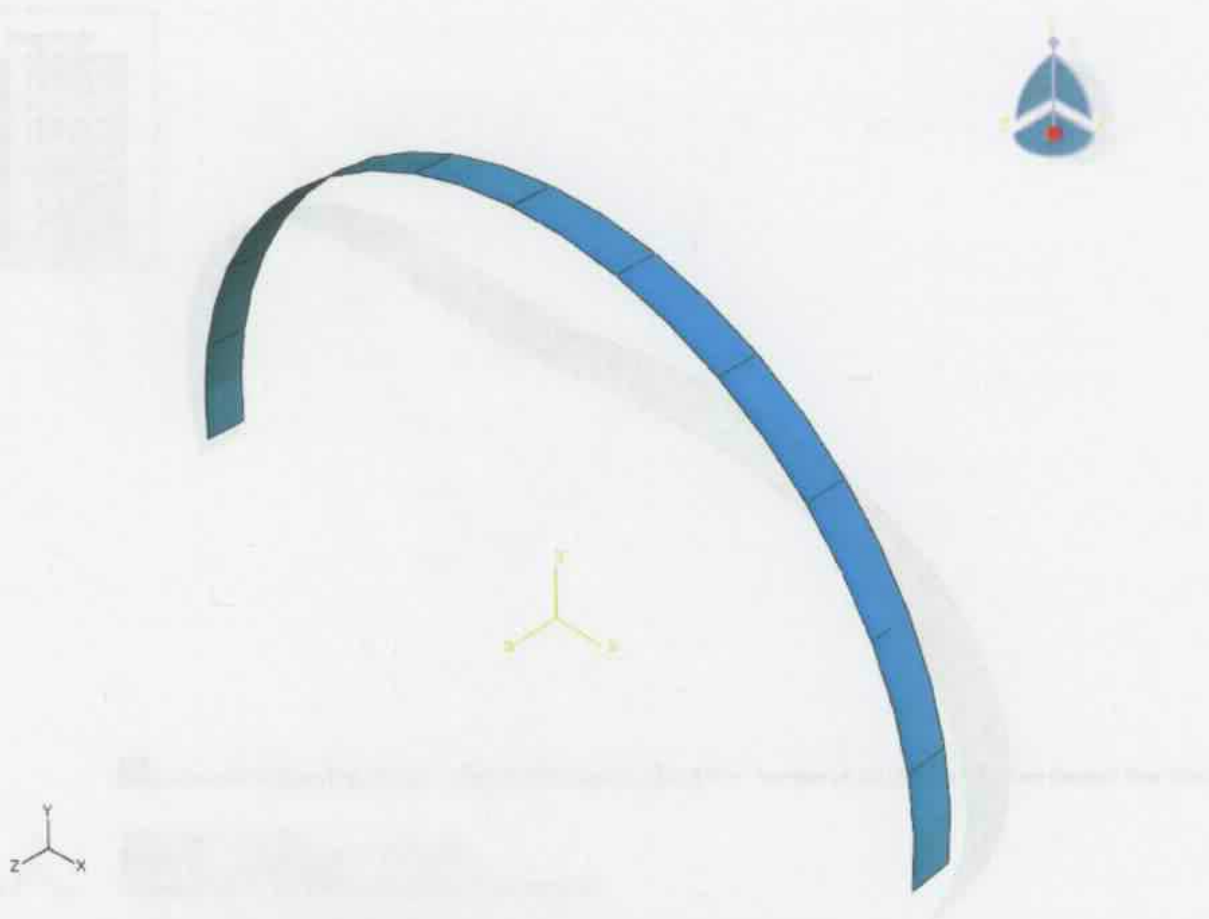
Figure 5.9b: Coarse mesh division of the arch.
