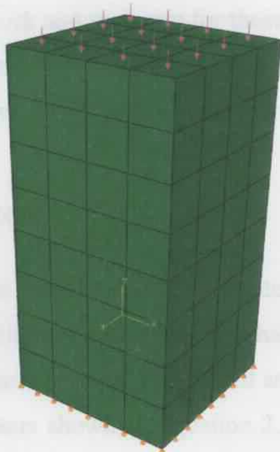
Figure 6.9: A uniaxial creep test.
