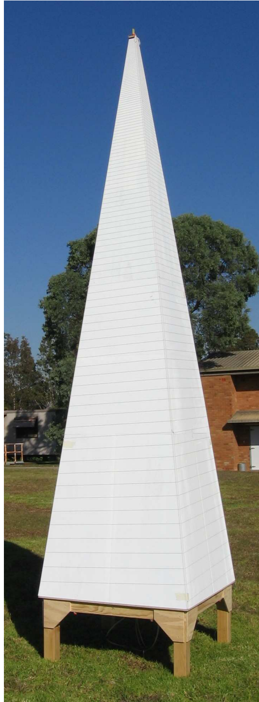
Fig. 4.1: The two arm, pyramidal, log-spiral antenna built for this work.
