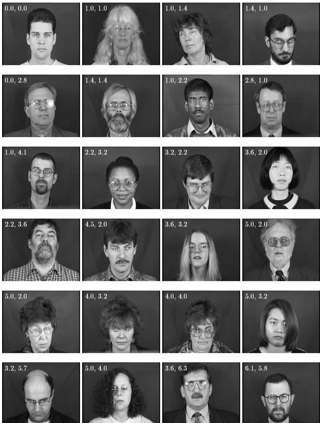
Figure 2.6: Results considered as good detections where both eyes are less than or equal to seven pixels away from the correct position. The top-left corner of each image displays the distances of the left and right eyes from the correct position, where the first number corresponds to the left eye and the second to the right eye.
