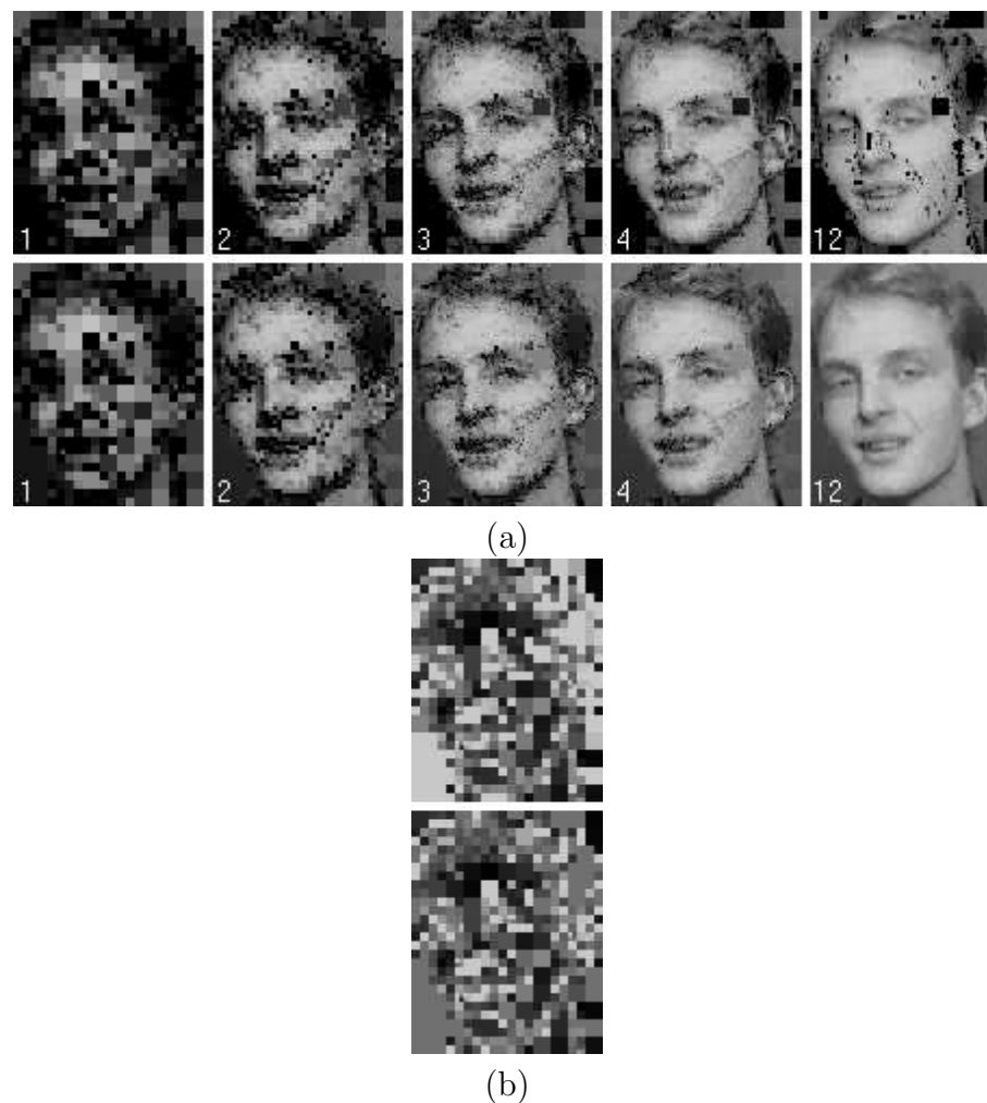
Figure 4.4: Comparison of results before and after \alpha modification to ensure convergence: (a) results of decoding with an initial black image using a fractal code with quad-tree partitions having a maximum contrast scaling factor of 1.2. The top row shows the results before \alpha modification. The bottom row shows the results after \alpha modification with the threshold set at 0.7 examined up to the first three iterations. The numbers on the bottom left corner of each image is the iteration number; (b) the intensities in these two images show the \alpha values for each range block. The top image shows the \alpha value distribution before the modification, and the bottom image is the result after the modification. The higher intensity blocks have \alpha values of 1.2. After \alpha modification some of these have changed to 0.7.
