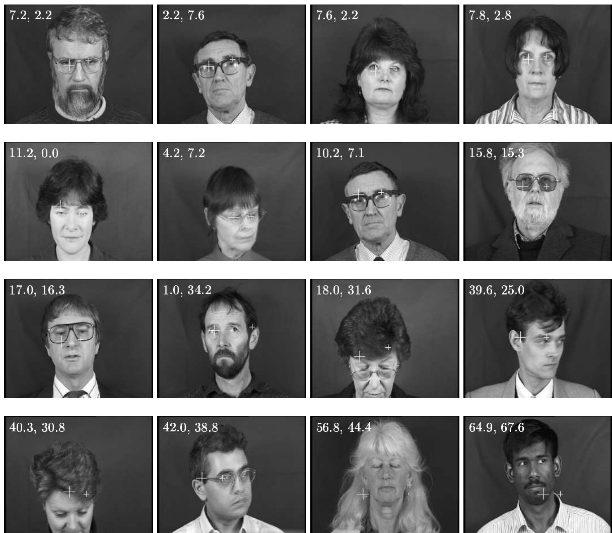
Figure 2.7: Results considered as bad detections where either or both eyes are greater than seven pixels away from the correct position. The top-left corner of each image displays the distances of the left and right eyes from the correct position, where the first number corresponds to the left eye and the second to the right eye.
