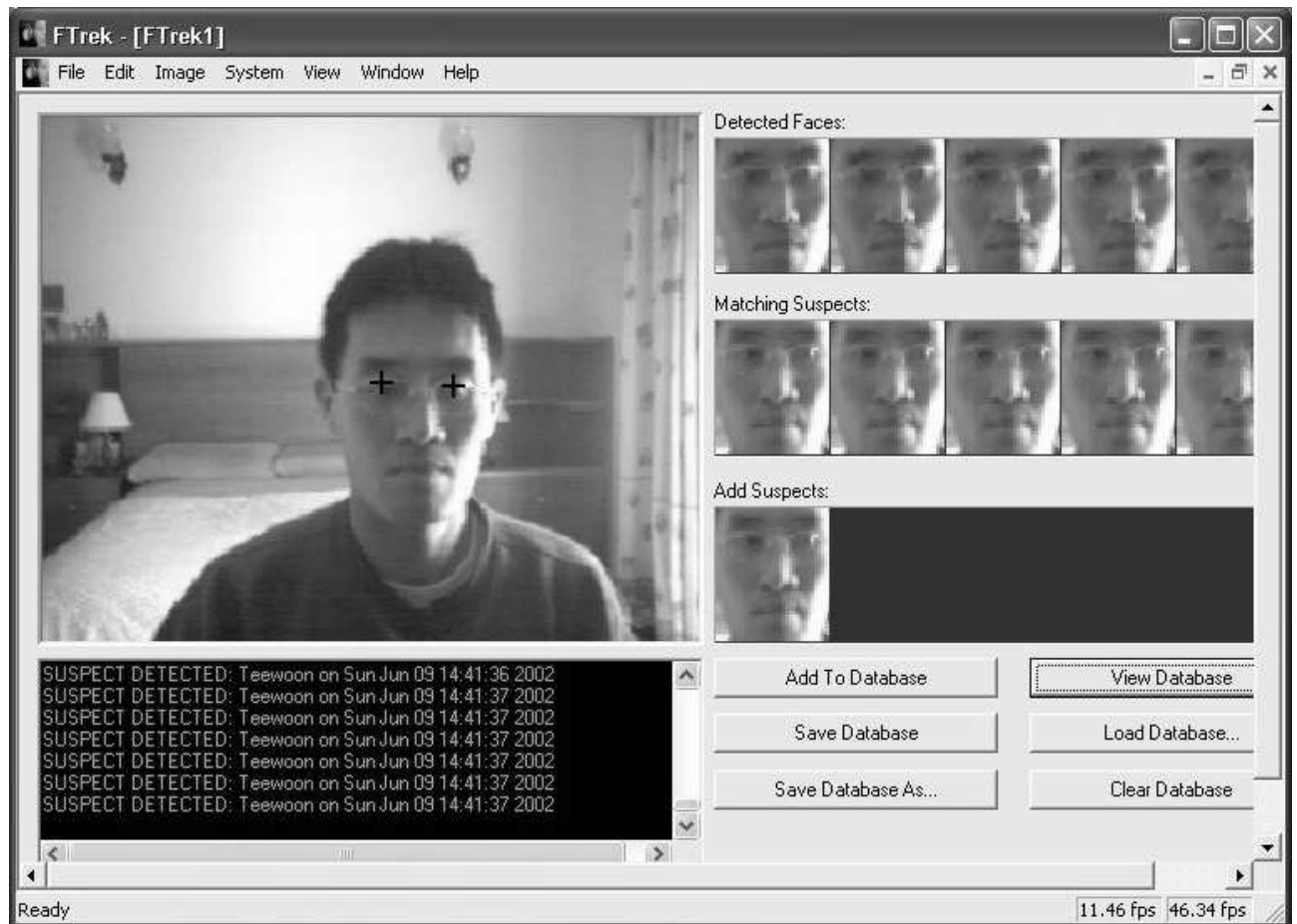
Figure F.1: User interface of the automatic face identification system. Detected eye locations are labelled using the '+' symbol. Extracted faces are shown in the row labelled 'Detected Faces'. Best matching faces in the database are shown in the row labelled 'Matching Suspects'.
