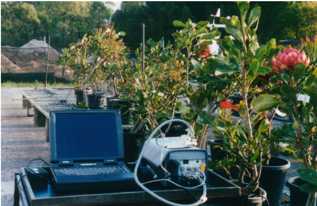
Figure 6.10: PAM 2000 fluorometer, for monitoring photoinhibition using chlorophyll fluorescence measurements, and laptop in use at Mount Annan Botanic Garden.
