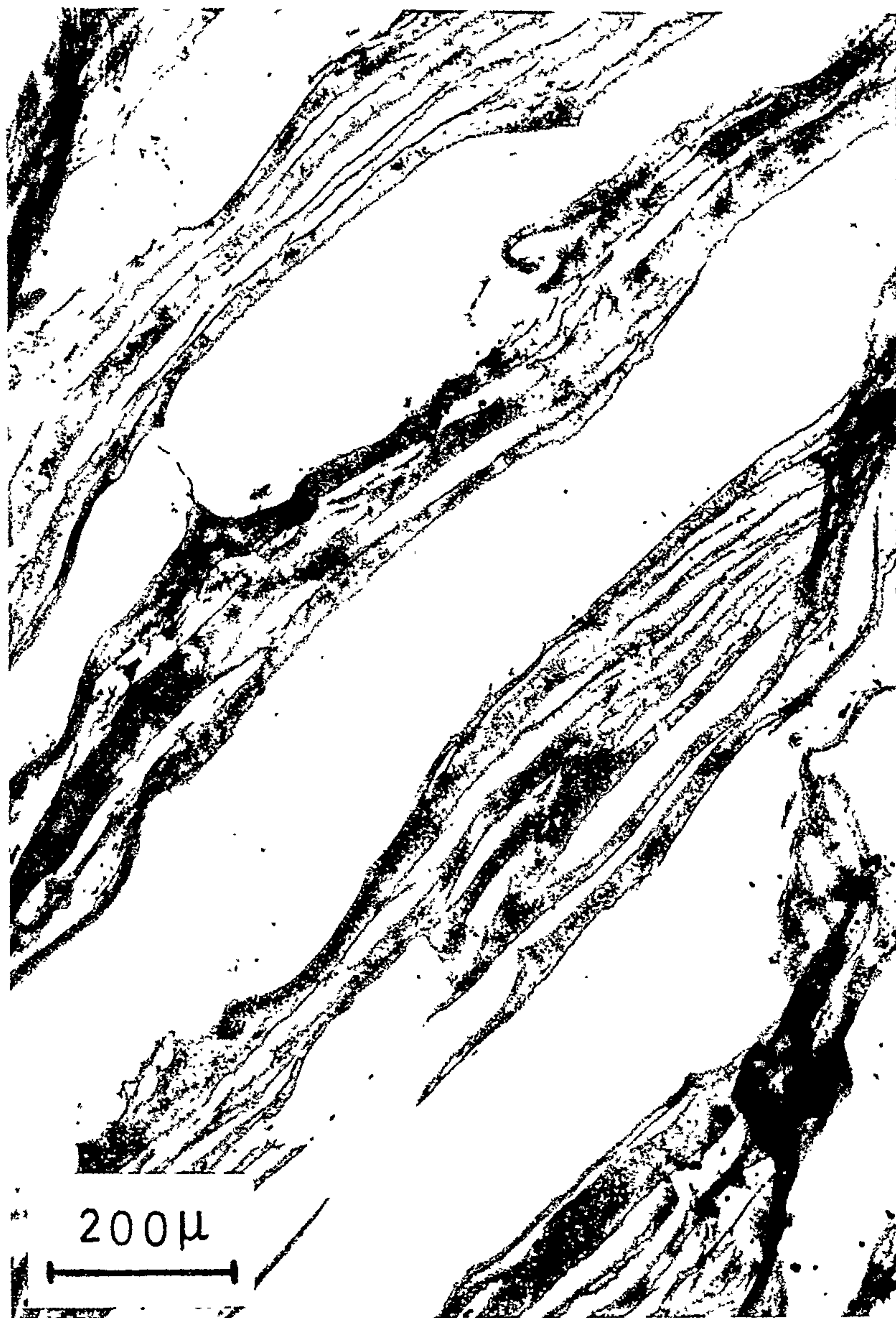
FIG. 16. Longitudinal section of cod muscle, showing both intracellular and extracellular ice in the same specimen. The effect was obtained by allowing partial cellular dehydration to occur by slow freezing, and then rapidly freezing to a low temperature, causing intracellular ice to form.
