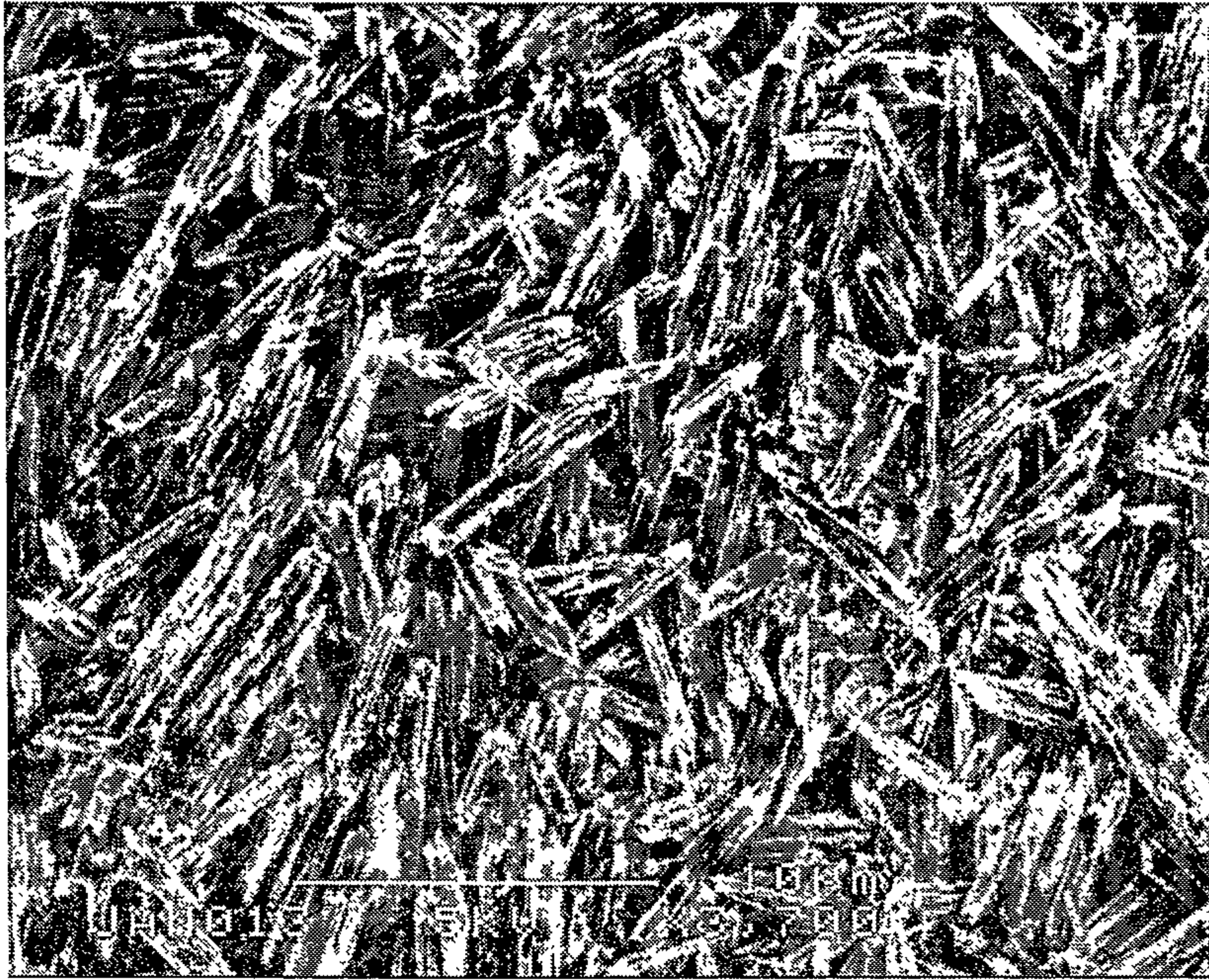
Figure 4.33 Lithium disilicate crystals in a bar-shaped specimen after repressing, where most crystals are aligned in the Y-axis direction, which is parallel to the pressing direction.
