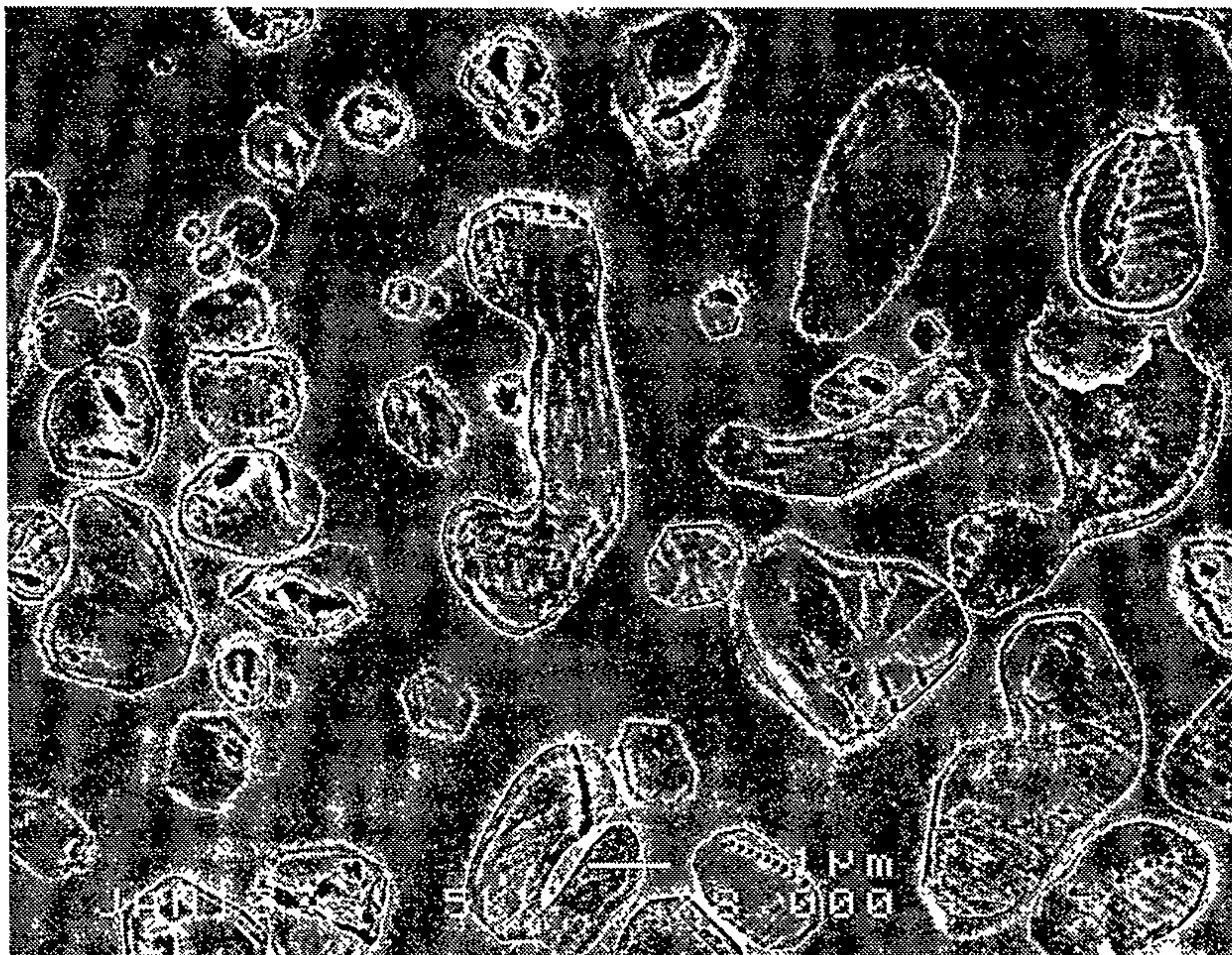
Figure 4.21 Extensive twinning of leucite crystals after pressing (magnification 8000 x).
