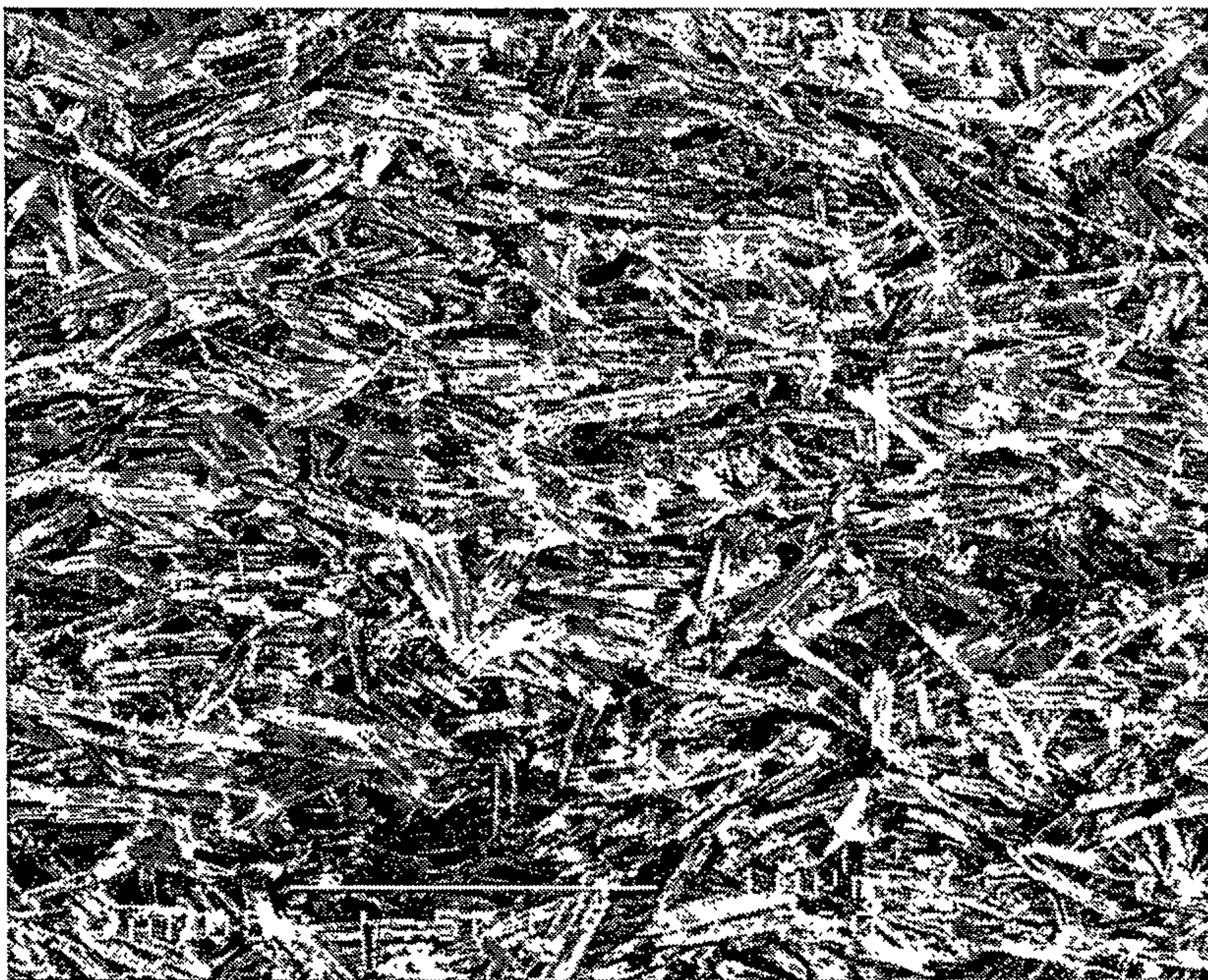
Figure 4.30 Alignment of lithium disilicate crystals in a sprue, where most crystals are oriented with their long axis parallel to the pressing direction (magnification 3700 x).
