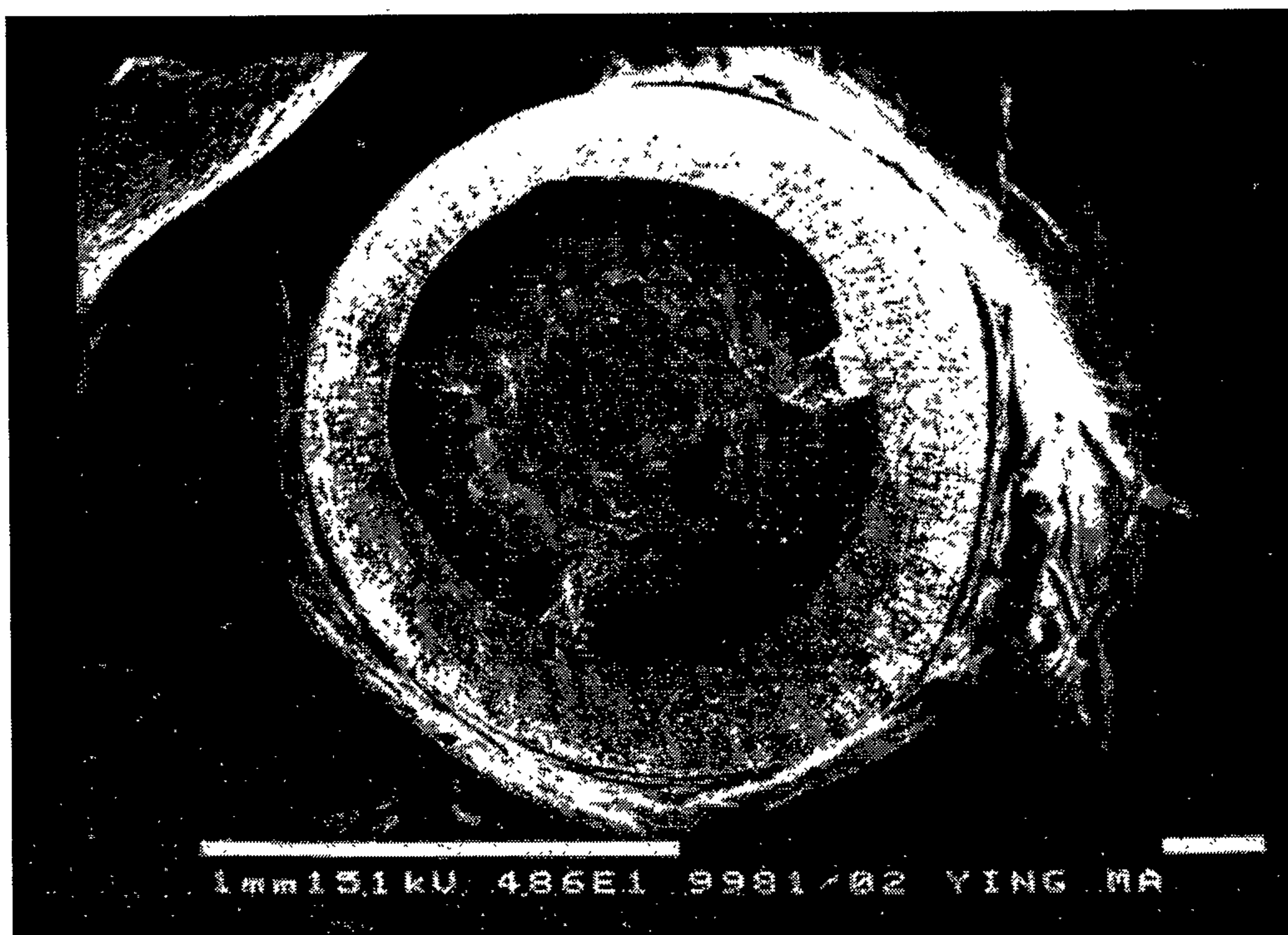
Fig. 3.20 Cross-section of tensile fracture part of WS wire.
