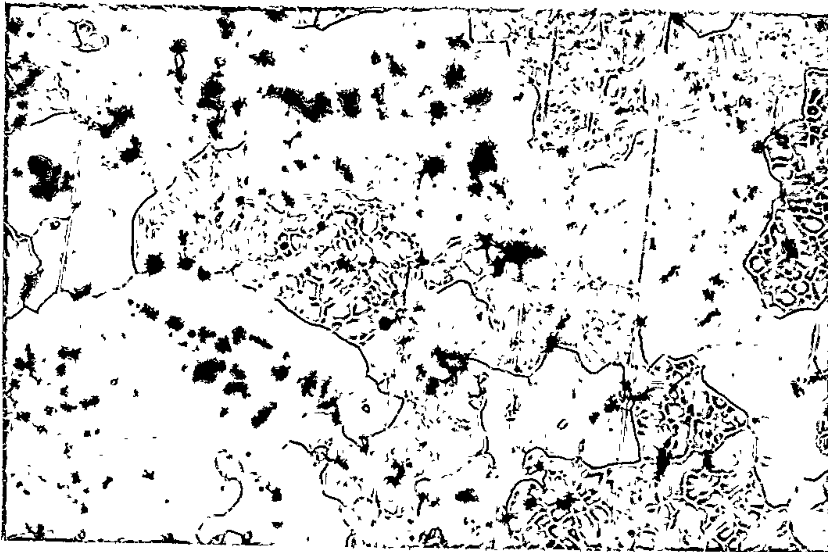
Precious Metal C Gold. (gas-air castings). X50.
