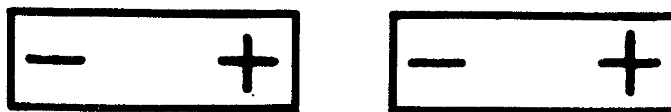
Fig. 3a Diagrammatic representation of Keesom forces – Orientation Effect
