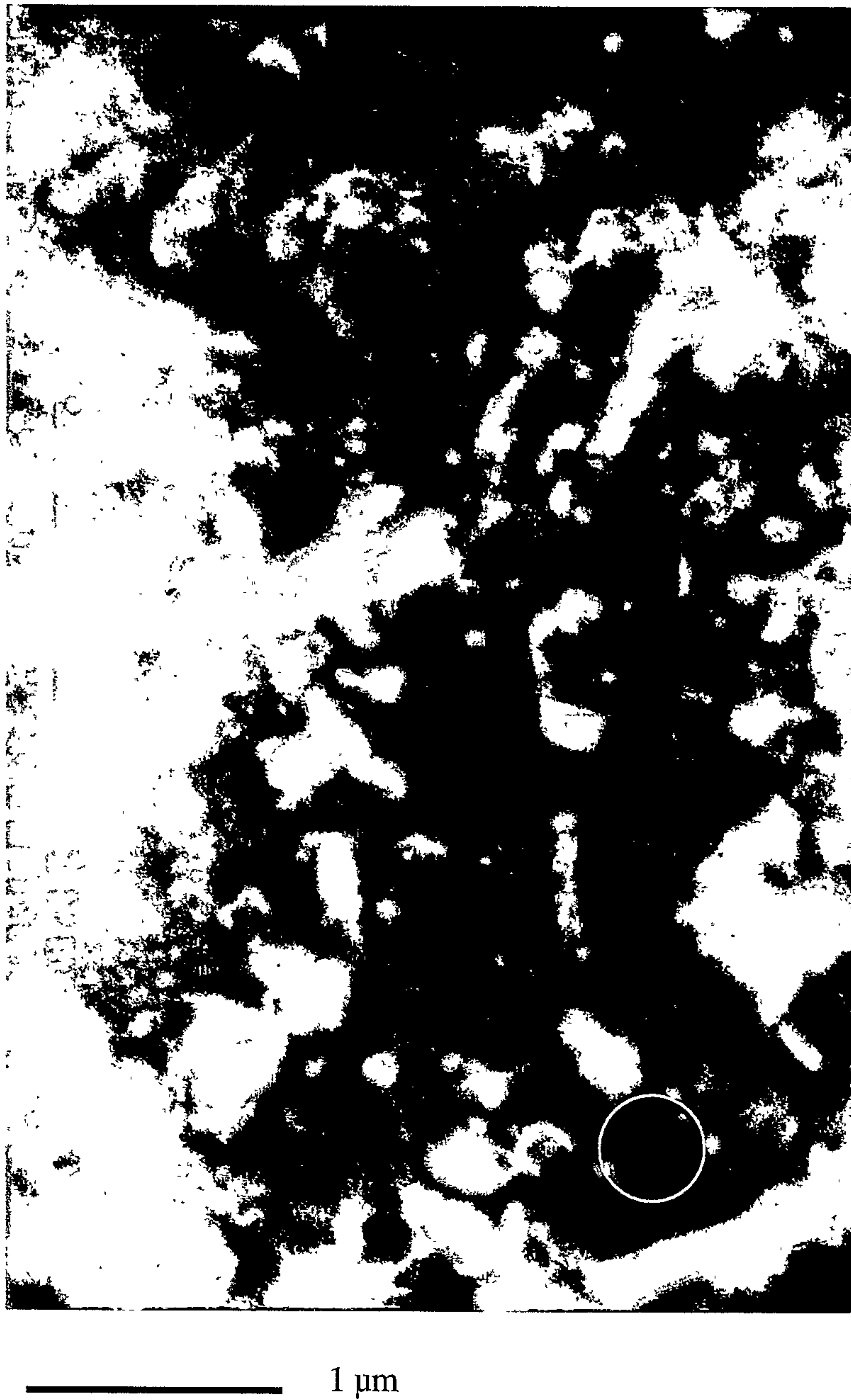
Figure 2.11 Scanning electron micrograph of the sintered alumina substructure of In-Ceram® after glass infiltration. This view of In-Ceram demonstrates the high saturation of the core with minimal porosity present. An example of a residual pore can be seen circled in the lower right corner of the electron micrograph. Original Magnification 25,000x
