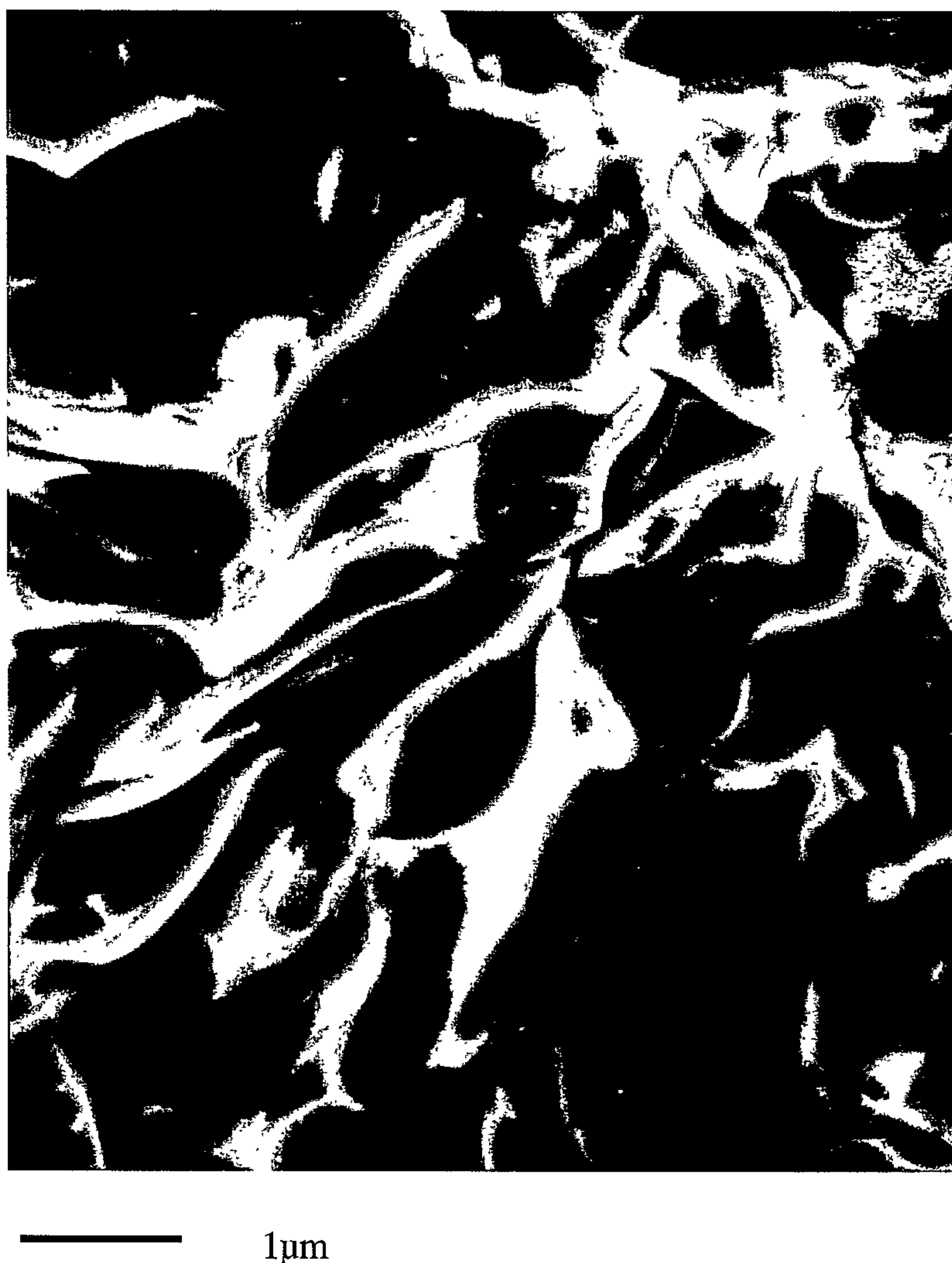
Figure 2.4 Scanning electron micrograph of a feldspathic veneering porcelain, Vitadur N®. Note the lack of distinct crystalline structure and the glassy appearance of this porcelain. Original Magnification 1000x.
