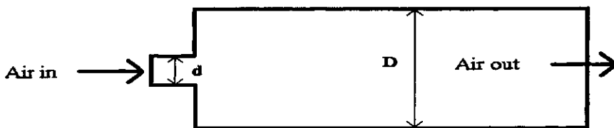
Figure 2.5 - Schematic diagram of sudden expansion. Source : Guo et al. (1998).
