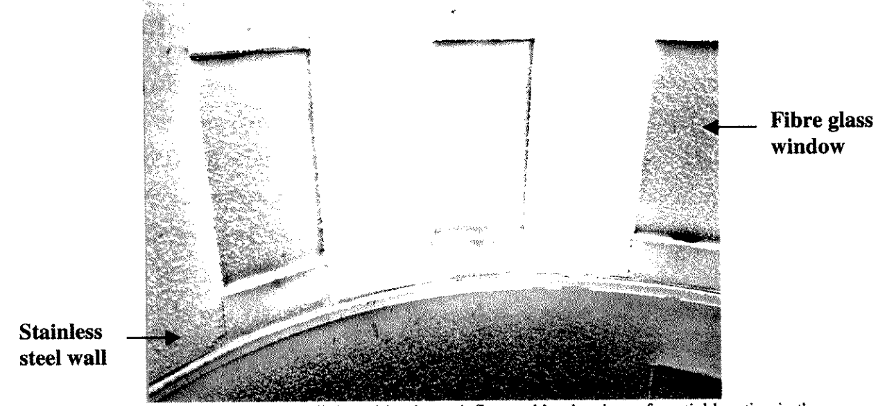
Figure 5.3 – Photograph showing that wall deposition is not influenced by the circumferential location in the spray dryer because the skim milk powder is evenly spread out.
