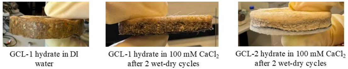
Figure 6.2. Representative photographs of GCL specimens after conditioning: (a) GCL-1 hydrated in DI water; (b) GCL-1 hydrated in 100 mM \text{CaCl}_2 and subjected to two wet-dry cycles; (c) GCL-2 hydrated in 100 mM \text{CaCl}_2 and subjected to two wet-dry cycles.
