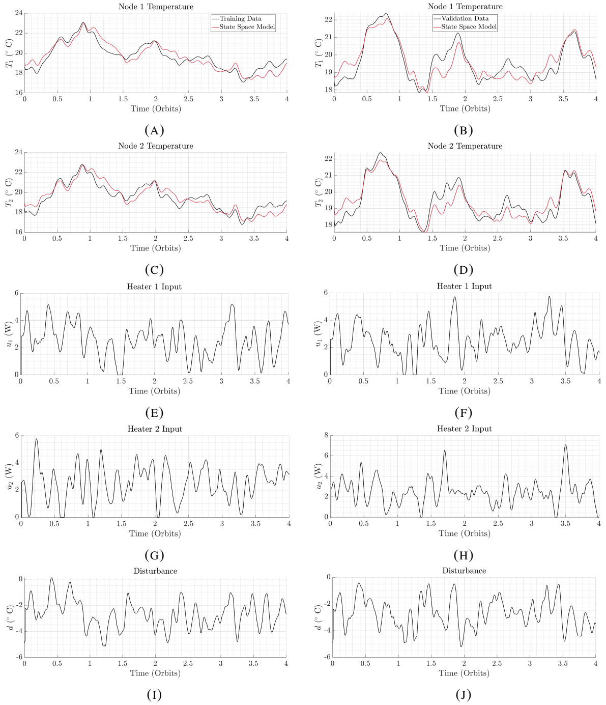
FIGURE A.1. System identification results for 7° inclination Cold Case orbit. Note all orbital cases were used in the fitting of parameters. Panels (A), (C), (E), (G), and (I) show the nodal temperatures, heater inputs, and disturbance inputs for the training data. Panels (B), (D), (F), (H), and (J) show the same results for a validation case.
