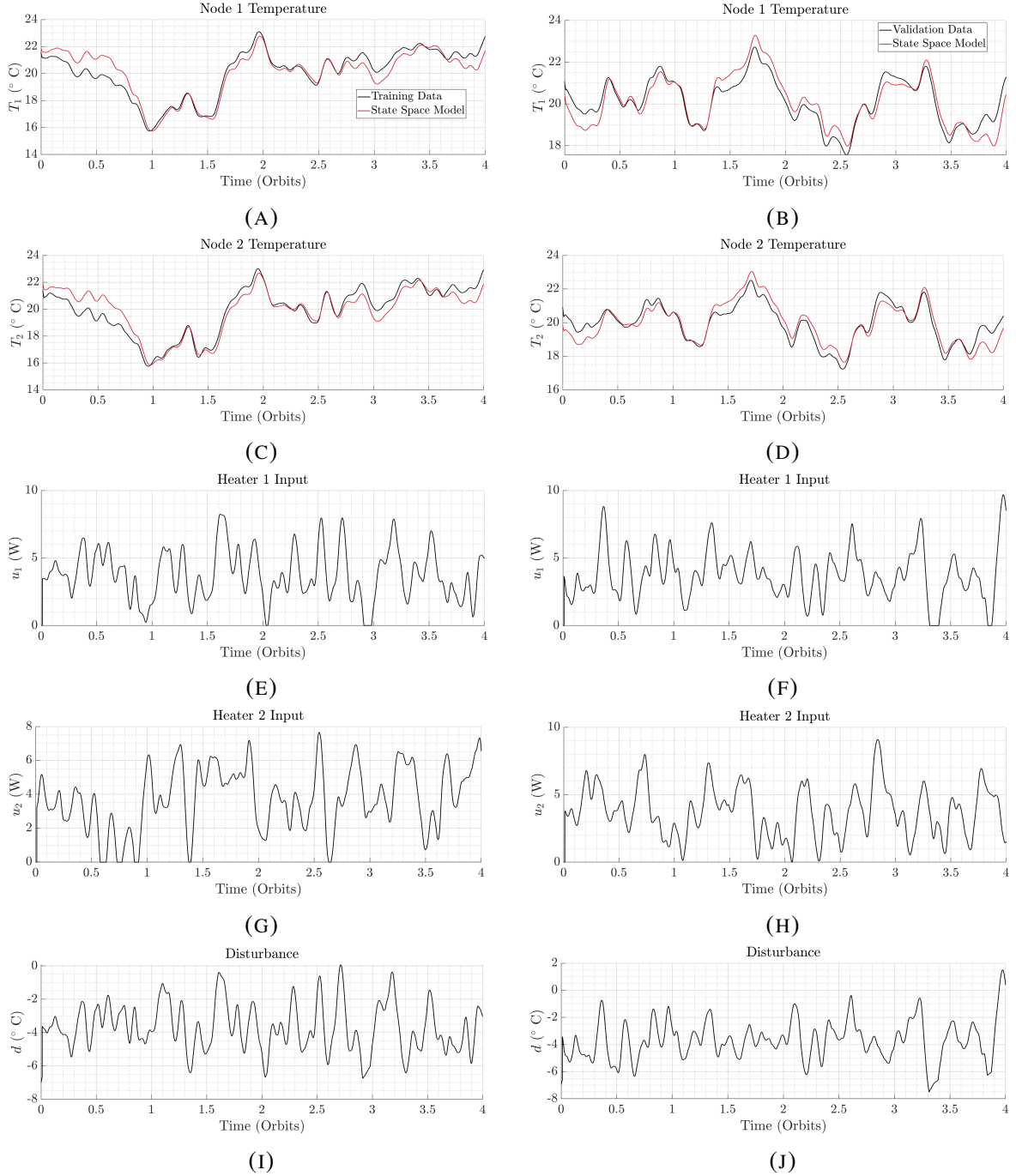
FIGURE 5.5. System identification results for 7° inclination Cold Case orbit. Note all orbital cases were used in the fitting of parameters. Panels (A), (C), (E), (G), and (I) show the nodal temperatures, heater inputs, and disturbance inputs for the training data. Panels (B), (D), (F), (H), and (J) show the same results for a validation case.
