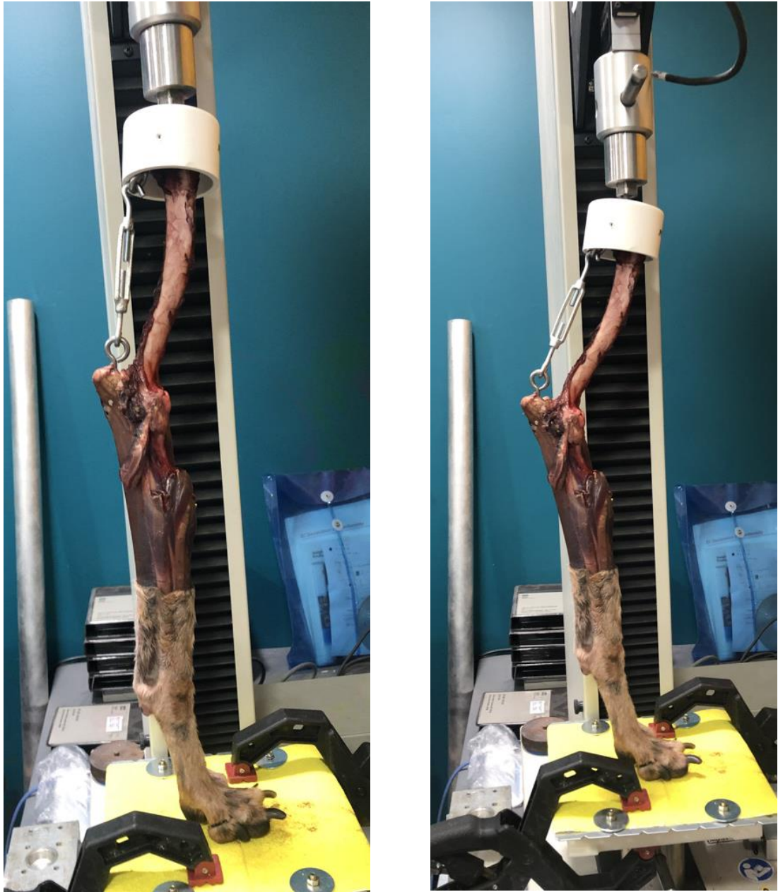
Figure 3.3.4: Photograph of limb mounted on materials testing machine.
