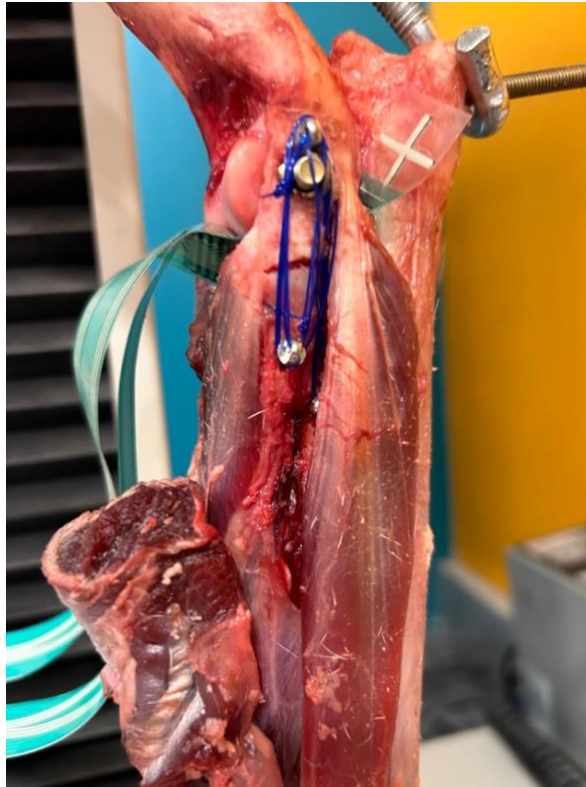
Figure 4.1.4: Lateral view of the elbow during testing, mounted on the MTS showing placement of the prosthetic lateral collateral ligament.
