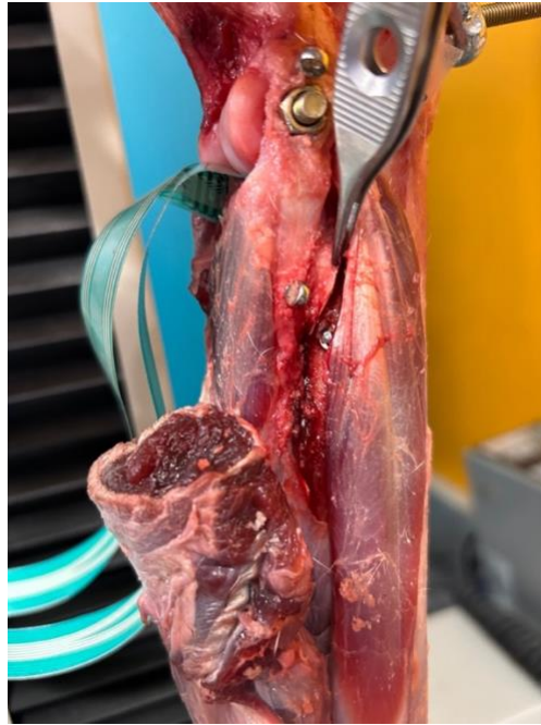
Figure 4.1.2: Lateral view of the elbow during testing, mounted on the MTS. Adson tissue forceps indicate where the cranial crus of the lateral collateral ligament has been transected.
