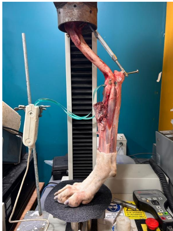
Figure 4.1.1: Alternate experimental set up with PCV cup replaced with metal cup.
