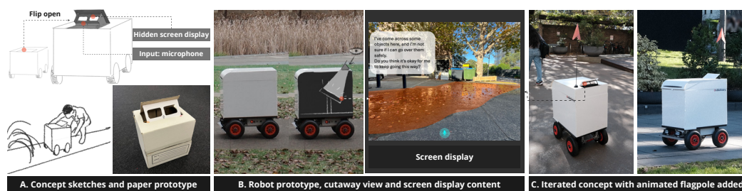
Fig. 9.1.: Concept development from initial sketches to final implementation: (A) Concept sketches, interaction illustrations, and a paper prototype in the early stage; (B) Robot prototype during the initial deployment, with a cutaway view and screen display content; (C) The iterated design concept featuring an added animated flagpole.
