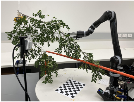
(c) Our laboratory setup mimicking the power line clearance scenario.
