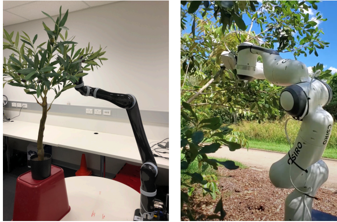
Figure 3.4: Experimental setup for robotic tree interaction. (a) Kinova Jaco-2 arm on synthetic plant. (b) Franka-Emika Panda arm on a real farm tree.
