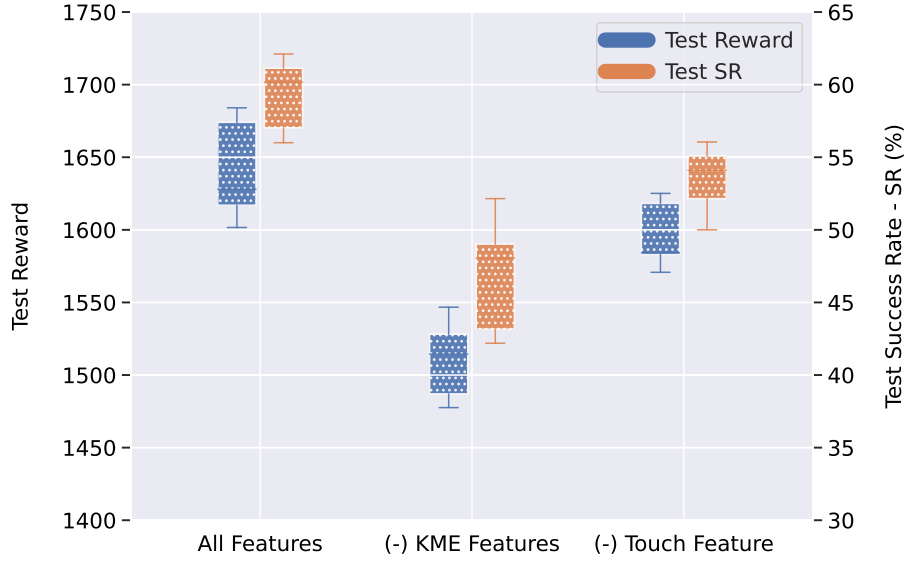
Figure 5.4: Ablation showing the relevance of key feature groups in our multi-modal policy. (-) indicates the removal of the single specified group. Each data point is a trained policy with a varying noise level. Boxes indicate median and IQR.
