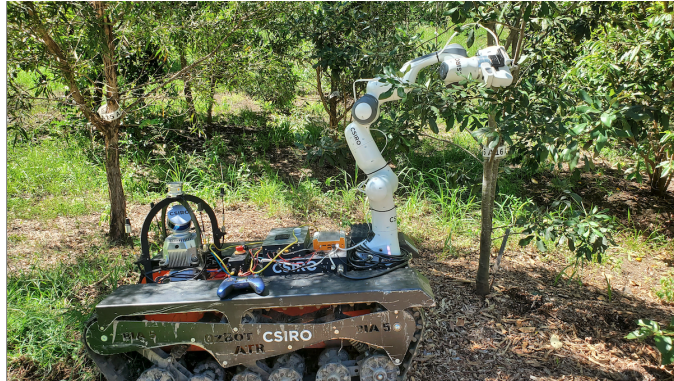
Figure 3.1: Autonomous navigation task: Our field robot obstructed by vegetation.
