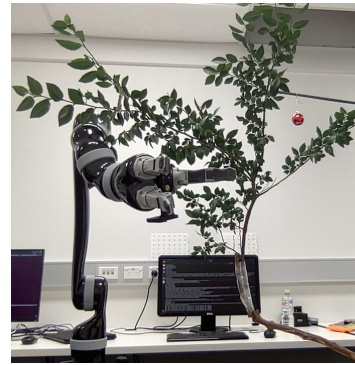
(c) Real setup: Kinova arm reaching for a previously unseen target (in red), obstructed by a real tree branch.
