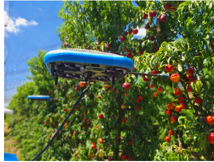
(b) An apple picking arm mounted on a drone, (Tevel, 2023).
