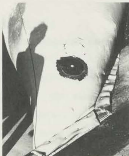
DIAGRAM 3.13 - A VIEW OF THE TAILORED END CLAMPING JUNCTION AND ASSOCIATED STRESS CONCENTRATIONS. THE PRESSURE RELIEF VALVE ENSURES PROTECTION AGAINST OVER INFLATION.
