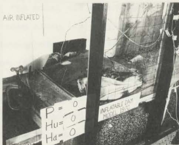
DIAGRAM 4.14 - COLLAPSED, DEFLATED BAG SHOWING FLEXIBILITY OF ENDS.
