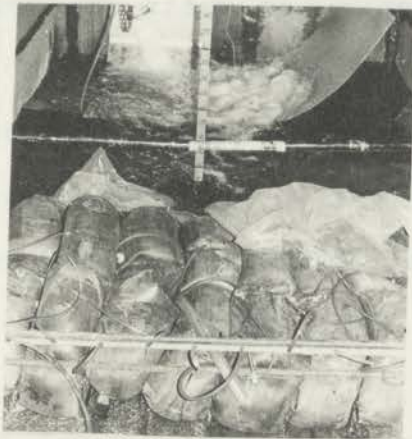
DIAGRAM 9.3 - WATER-INFLATED UNDER LOW INTERNAL HEAD, U/S HEAD = 0.8 FT - VERY LITTLE LEAKAGE.
