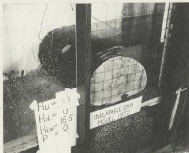
DIAGRAM 4.16 - A WATER-INFLATED CASE WITHOUT TRIP-WIRE. COMPARE THE SQUAT SHAPE OF THE WATER INFLATED CASE TO THAT OF AIR. ALSO NOTE THE TURBULENCE FREE WATER AND THE LOCATION OF THE STRAIN GAUGES ON THE DOWNSTREAM FACE. THE OVERFLOWING WATER IS SEEN TO CLING TO THE DOWNSTREAM FACE.
