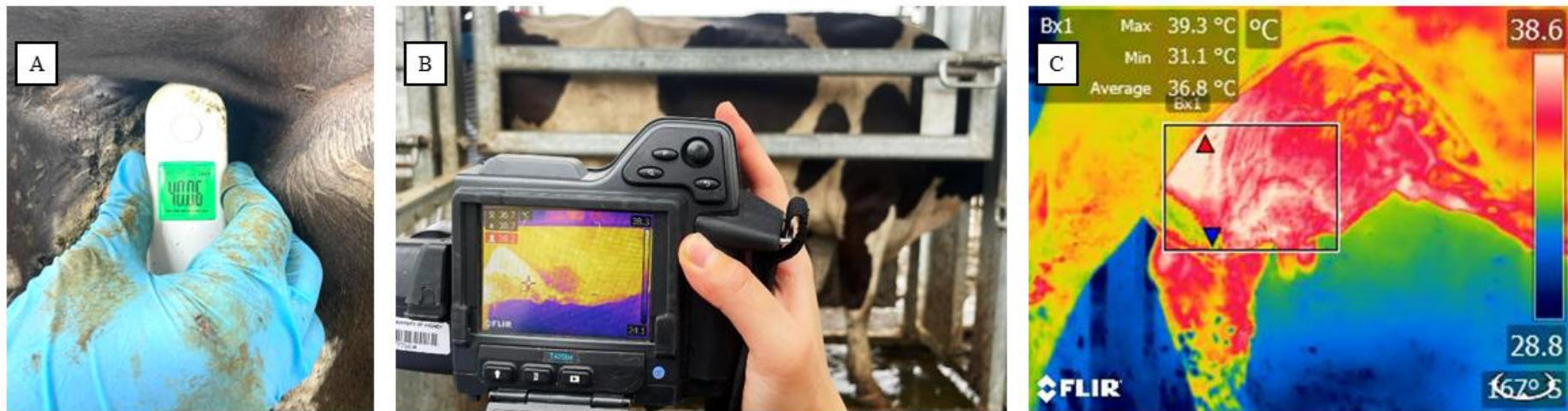
Figure 2. A) Rectal temperature measurement using a digital veterinary thermometer. B) Infrared image captured with a FLIR T420bx camera. C) Infrared temperature extraction using FLIR software; within each outlined rectangle, the solid red triangle indicates the maximum temperature (hottest point) and the solid blue triangle indicates the minimum temperature (coolest point).
