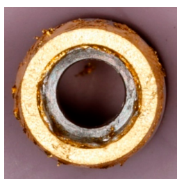
Figure 1. This image shows the fitting surface of a milled cobalt chrome abutment after the application of a 23-karat gold 0.12 µm foil layer. The gold foil is manually adapted to the connection geometry prior to assembly and subsequent microleakage testing.
