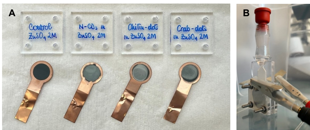
Figure 4.19A: The round shaped Cu electrodes after the zinc plating experiments, and B: transparent 3D-printed asymmetric Zn||Cu cells configuration.
