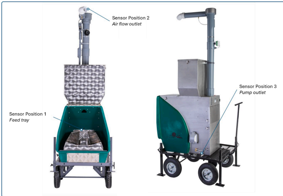
Fig. 4. Locations where the low-cost experimental gas sensors were positioned on the GreenFeed unit.
