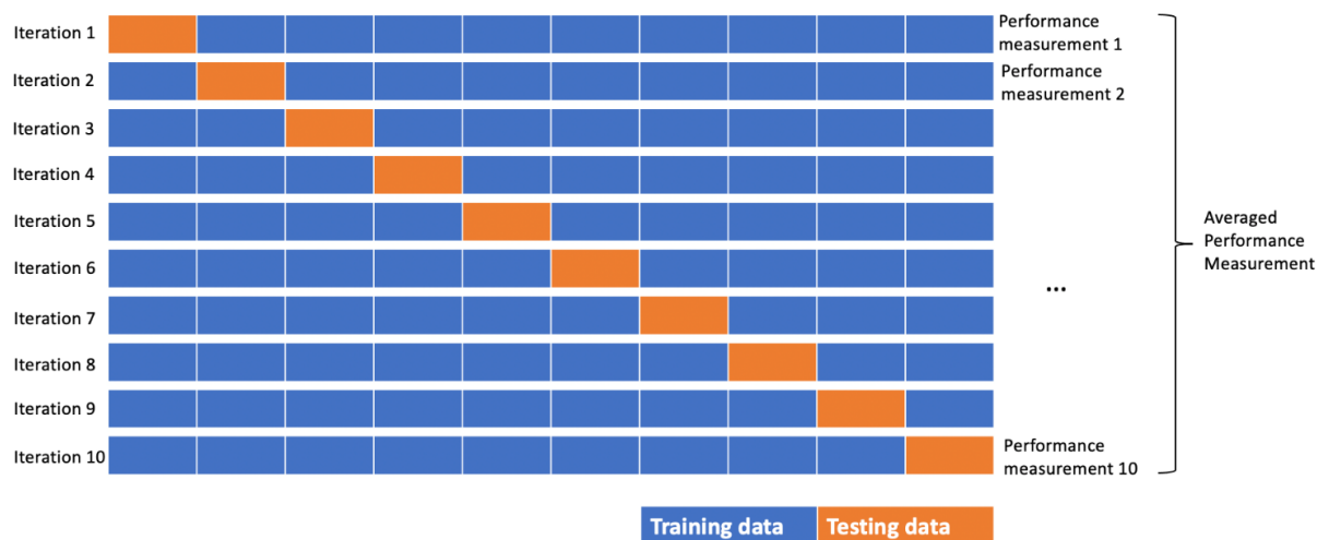
Figure 3.10 Demonstration of 10-fold cross validation. The dataset is divided into 10 equal-sized subsets (folds). In each iteration, one fold is used as the testing set, while the remaining nine folds are used for training. Performance metrics are computed for each iteration, and the overall model performance is obtained by averaging the results across all folds.
