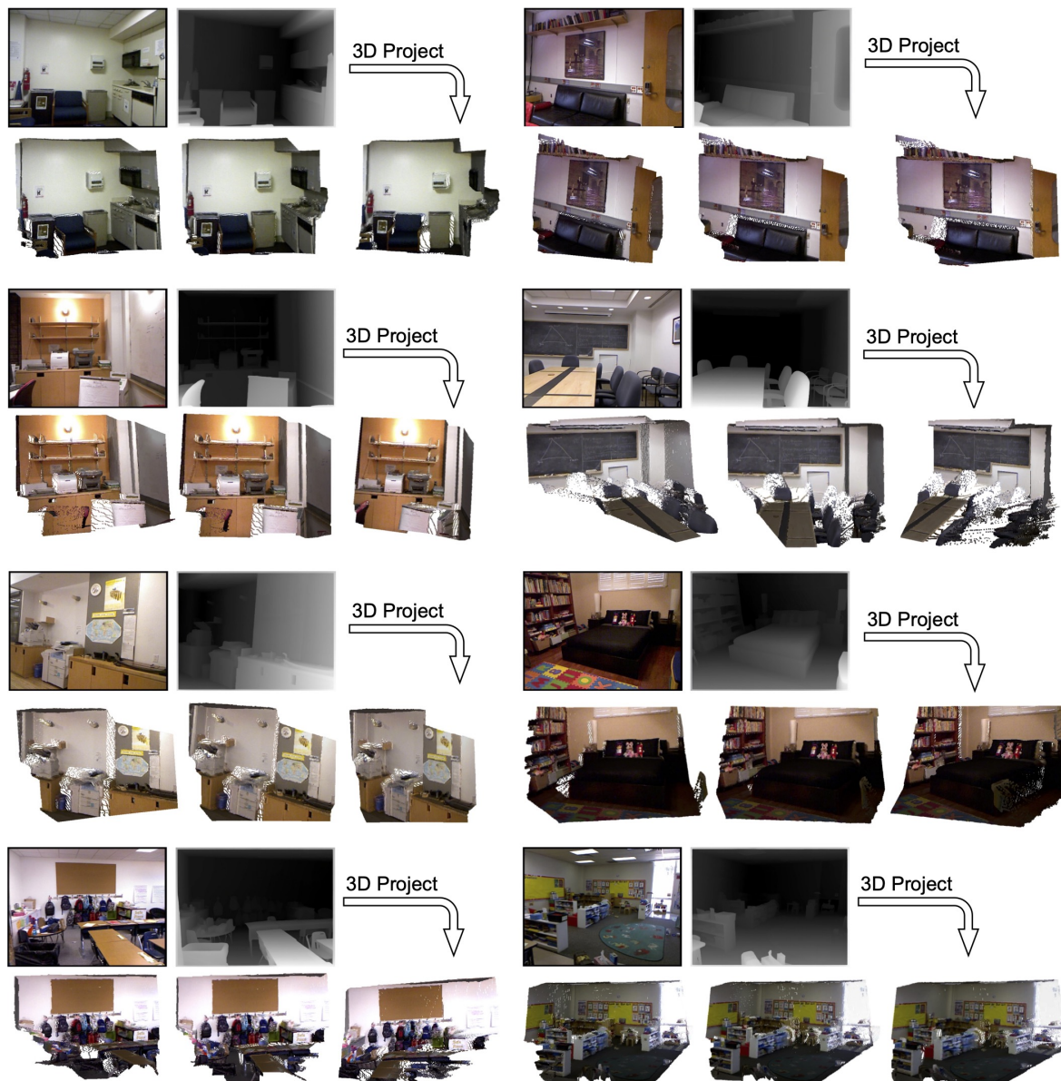
FIGURE 4.20. Potential application of single-view scene reconstruction. Given an RGB image and predicted depth map, we lift this image into a 3D space. We illustrate three views of this scene. Best viewed in color.
