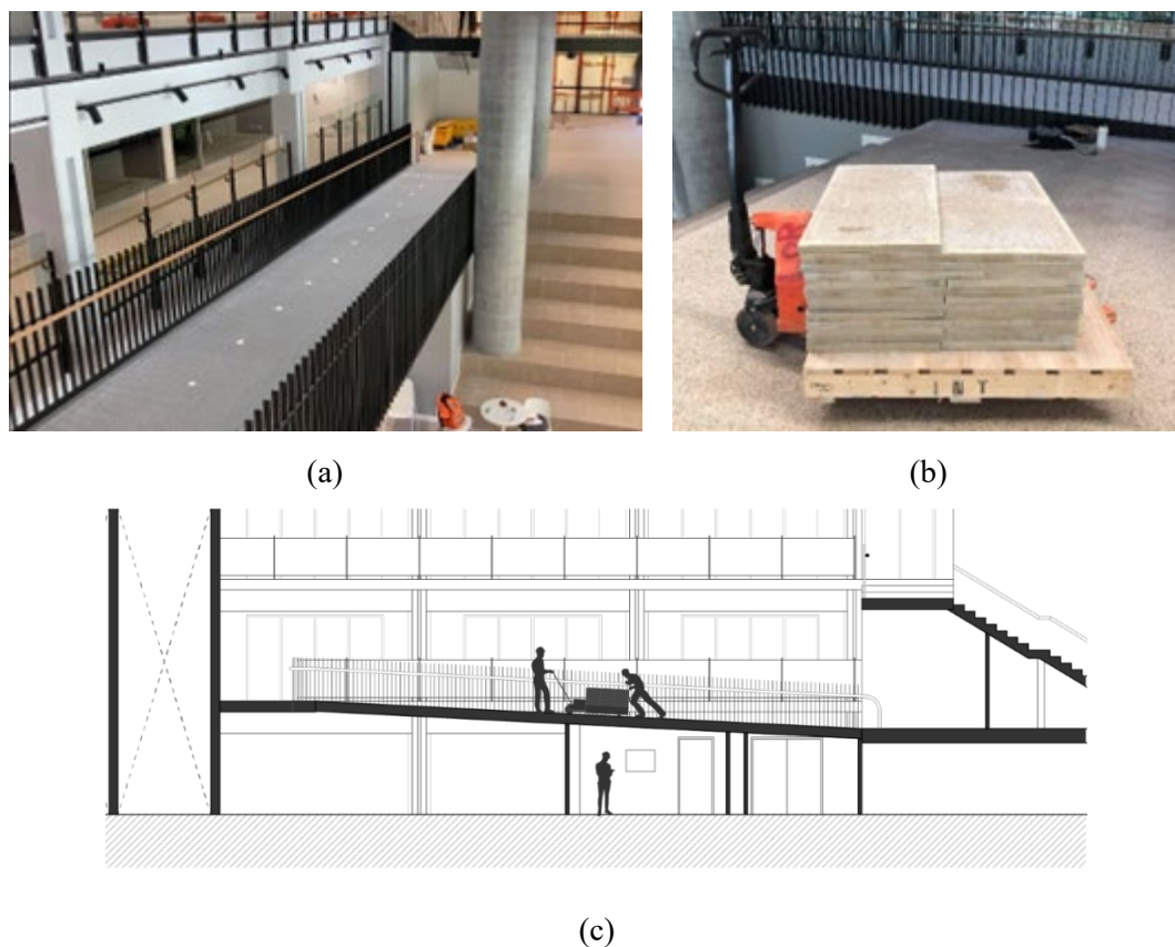
Figure 6.4 – (a) Footbridge with marked FBG locations, (b) pallet crate load, and (c) section of experiment
