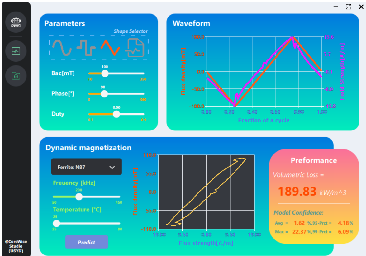
FIGURE 6.4: User interface for single-cycle prediction, showing input waveform, B – H loop, and core loss results.
