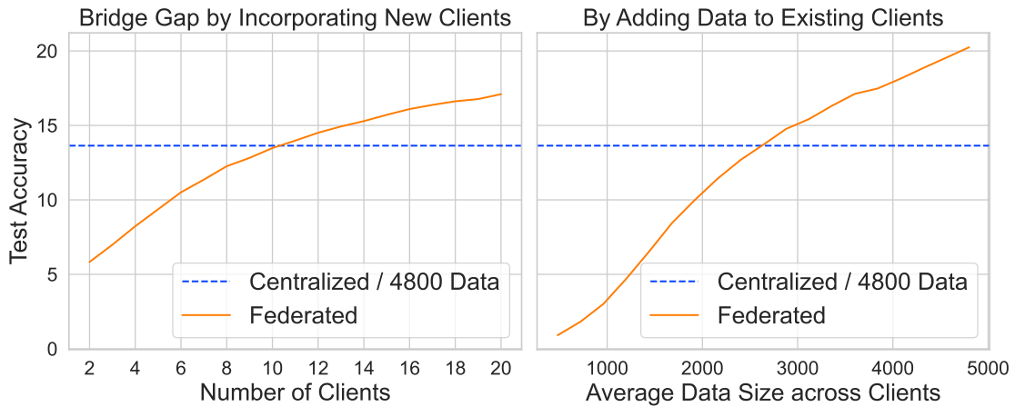
Figure 4.4: Empirical evidence for fully closing the gap between federated and centralised training setups. (Left) The strategy of incorporating new clients (increasing the number of clients n ). (Right) The strategy of adding data to existing clients (increasing the average data amount m ).
