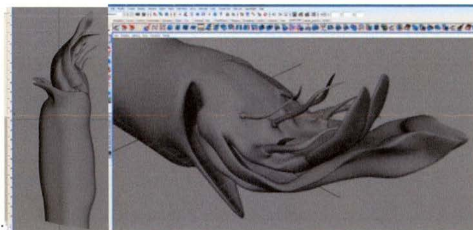
Figure 106 Screen shots of the Pyeganelia stricta . The software was better suited for the making of organic shapes and delicate detail. This was achieved using either 3DSMAX or MAYA software, which are normally used for animation, not for making solid objects.
