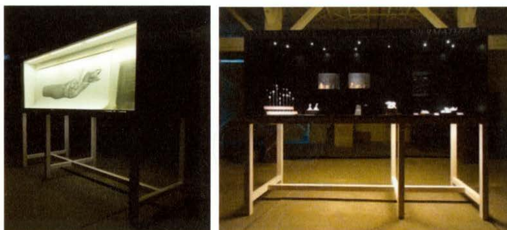
Figure 126 White back, flat light, for contrast for print displays. Front of cases was painted black inside and out, and LED light was pointed at small objects alone, through 4-8 mm holes cut out in circles or rectangles depending on the object to be lit.
