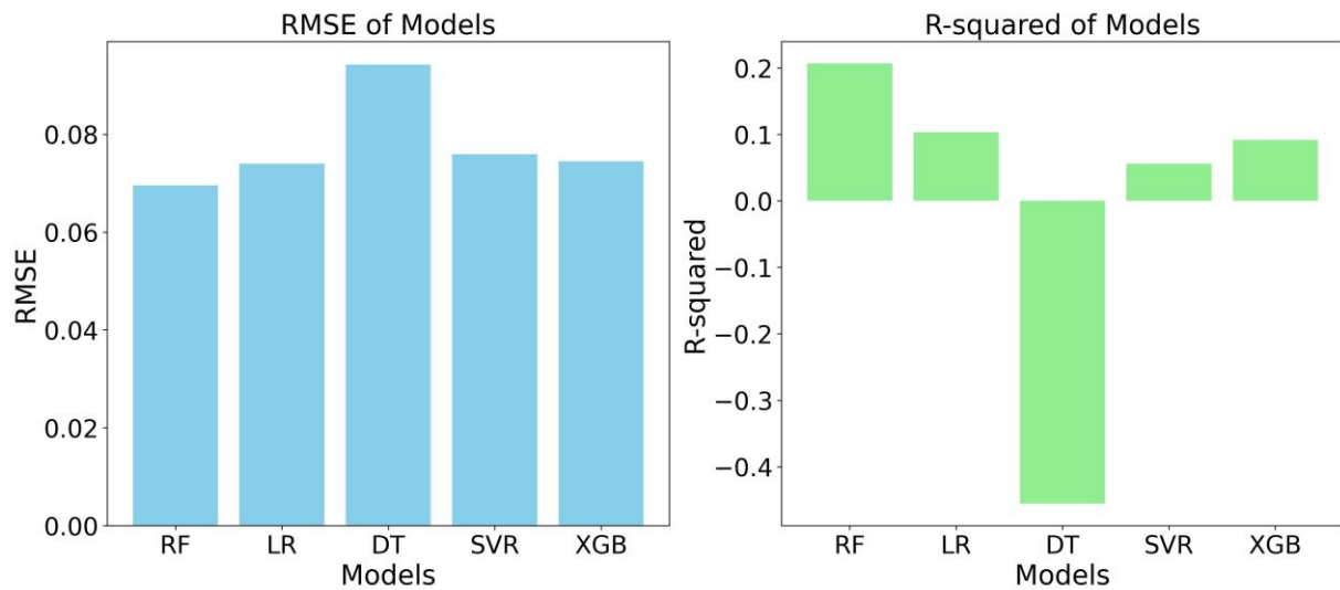
Fig. 14 (a) Pearson correlation coefficients of variables used in the model with topsoil thickness measurements, (b) variable importance in modeling topsoil thickness, (c) Comparison of different machine learning models (RF: Random Forest, LR: Linear Regression, DT: Decision Tree, SVR: Support Vector Regression, XGB: XGBoost) for predicting topsoil thickness.
