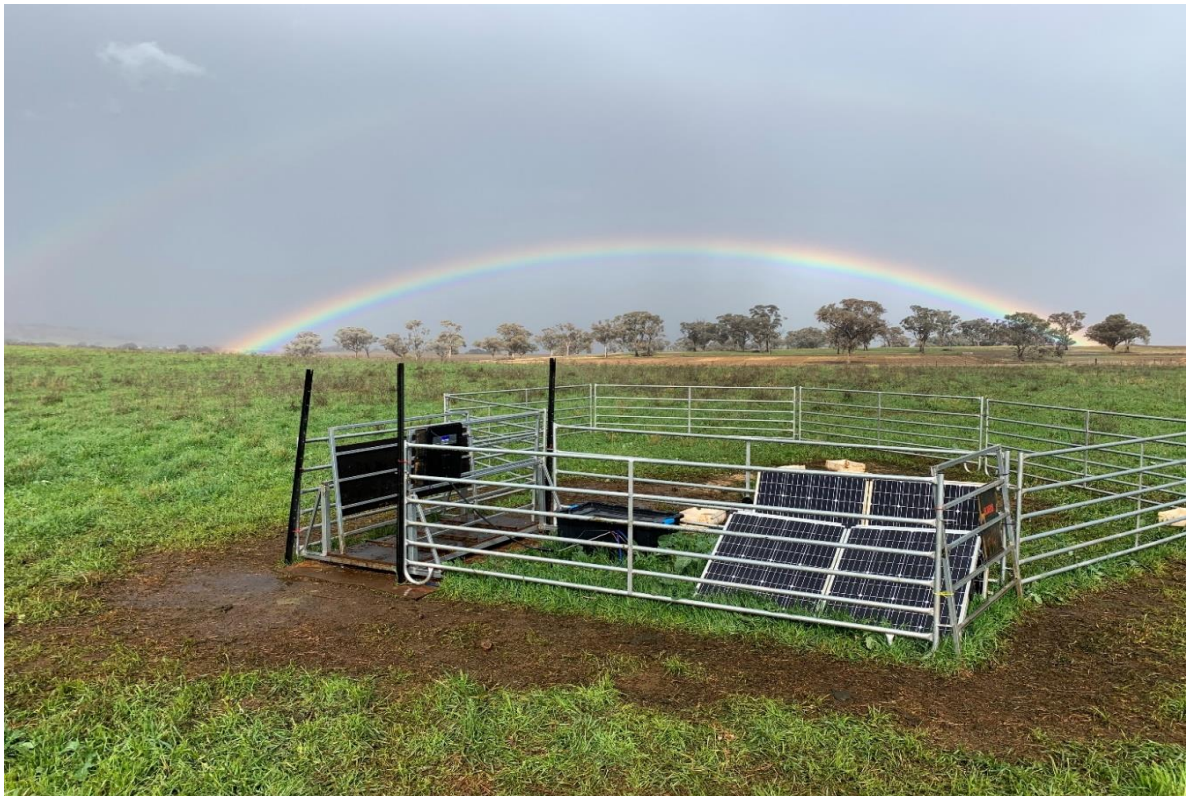
Figure A.3. walk-over-weighing platform that requires lifting on to a trailer and dismantling before moving to another paddock.
