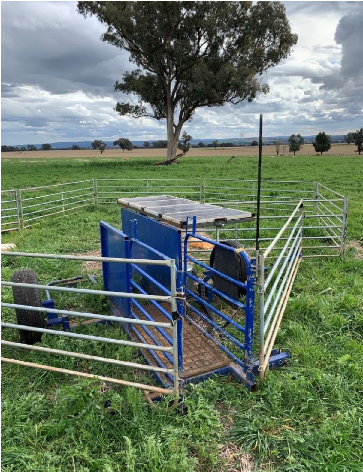
Figure A.1. walk-over-weighing platform that can be towed from paddock to paddock and set up as a complete unit.
