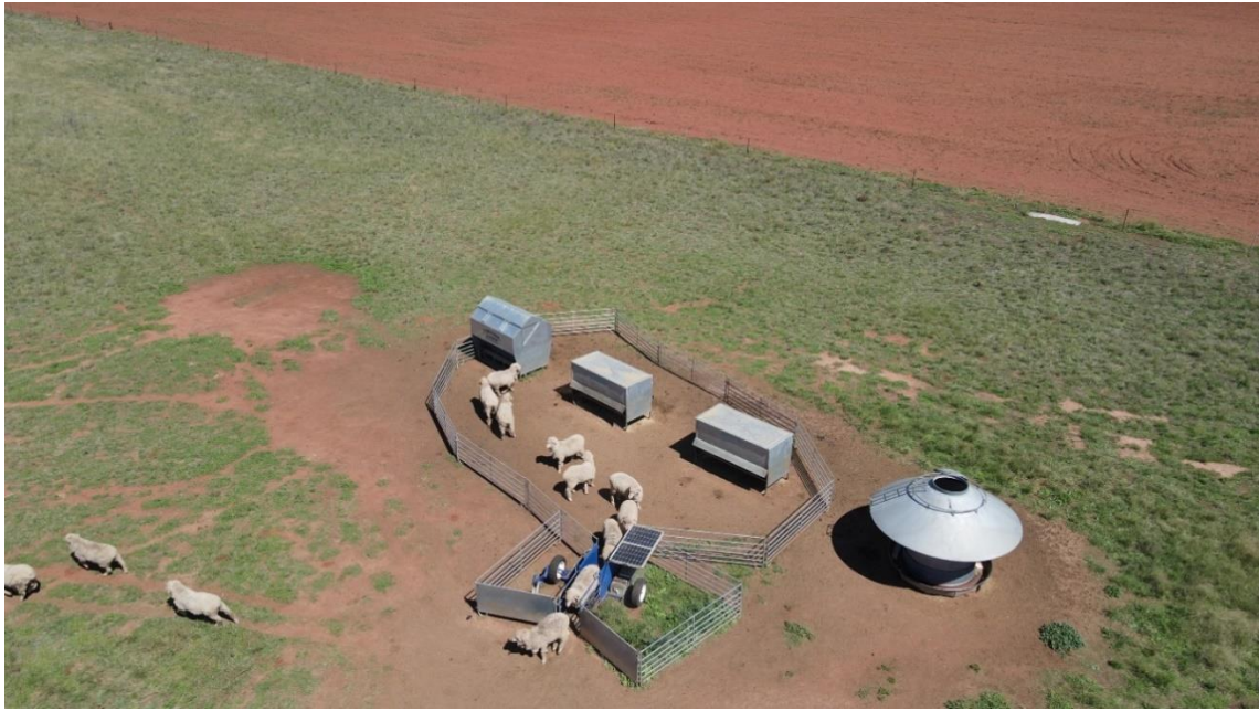
Figure A.2. Birds eye view of the transportable walk-over-weighing platform with merino rams traversing.
