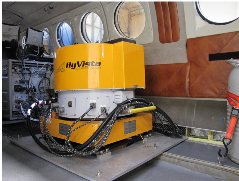
Figure 2.4: The HyMap device developed by HyVista Corporation has been employed by many Earth-observation studies[75].
