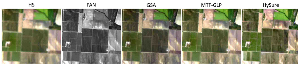
Figure 2.5: Schematic showing the increased ground sampling afforded by various pansharpening techniques[98].
