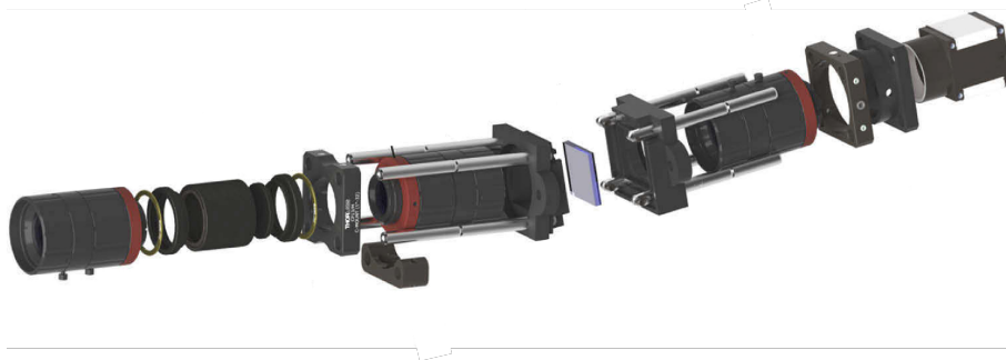
Figure 2.3: Exploded view of the Henriksen et al. V6 DIY spectrometer. Figure adapted from Ref. [61]
