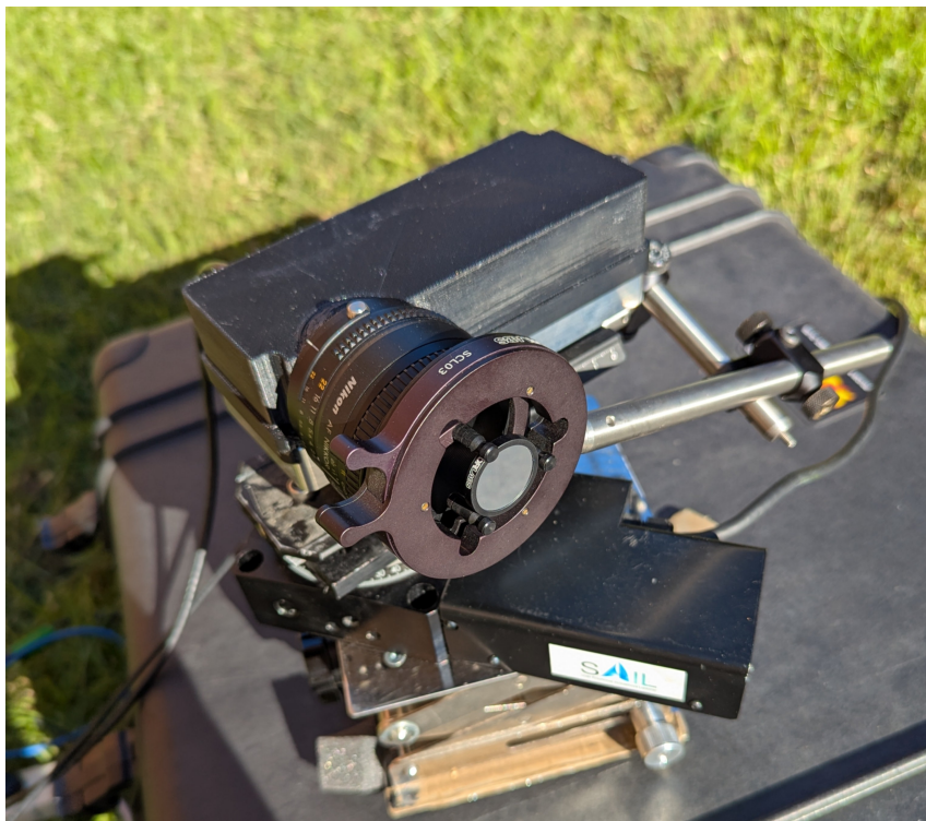
Figure 6.19: Multi-spectral panchromatic image capture setup showing the small circular filter held in place in front of the field lens.
