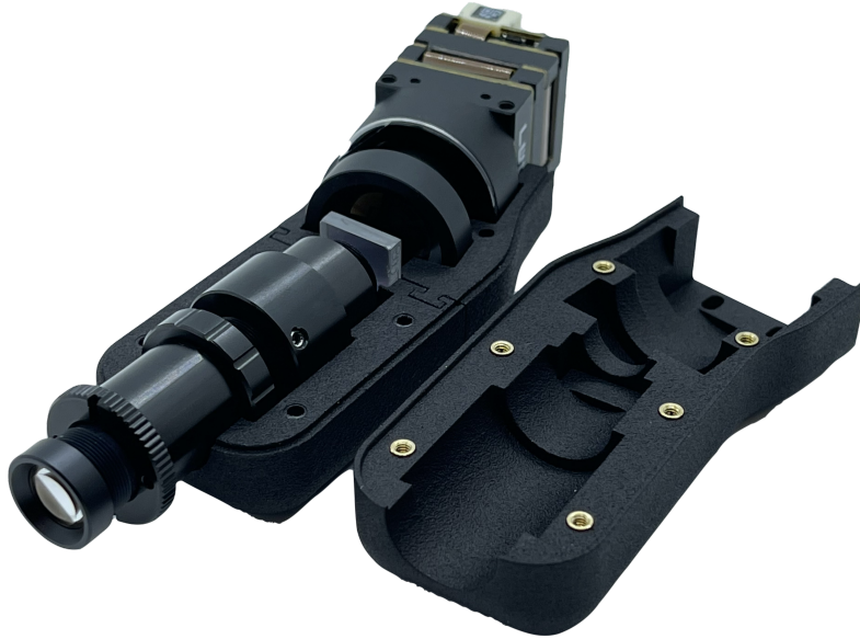
Figure 4.1: A physical Openhsi model showing 3D-printed two-part housing and small field optics for portable applications.
