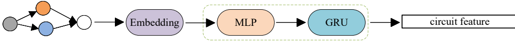
FIGURE 4.3. The pipeline of the GNN-based encoder. The block ‘Embedding’ represents an embedding layer that can transform the discrete node information to a continuous vector. The block ‘MLP’ is a multi-layer perceptron and the block ‘GRU’ refers to a Gated Recurrent Unit.
