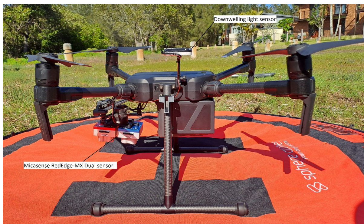
Figure 3. The DJI Matrice 200 UAV used in this study. The Micasense RedEdge MX Dual camera system and the downwelling light sensor are labelled. Photo by Jamie Simpson.
