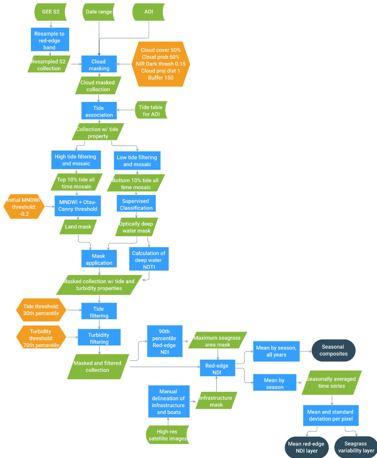
Figure 2. Flow diagram of full processing workflow applied to filter and mask Sentinel-2 image collection to remove cloud and select low tide and turbidity images, calculate the maximum seagrass area, and generate seasonal composites and seasonally averaged time series.
