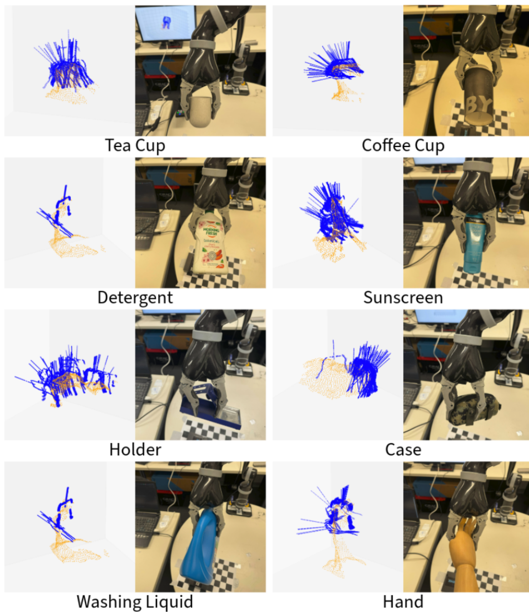
FIGURE 4.8. The picture on the left illustrates fifty grasp poses generated with the same point cloud. The photo on the right is the actual grasp for one of the five grasps in Table. 4.4. Our algorithm can grasp objects with large occlusions and noisy point clouds.
