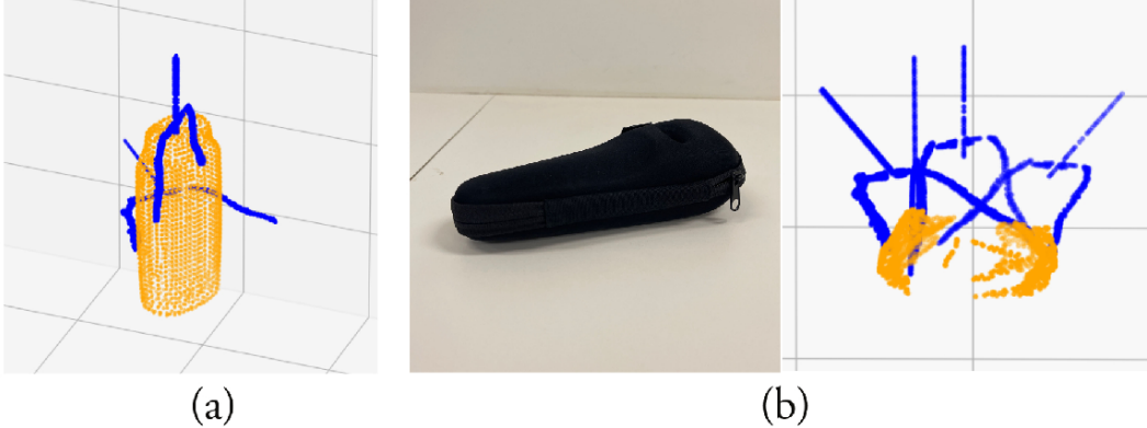
FIGURE 3.5. (a) Both grasp poses are successful, but a configuration with a smaller opening between fingers would provide a better grasp. (b) The case where occlusion is too large leading to failure due to collisions. It demonstrates a limitation of our algorithm in dealing with significant occlusions.
