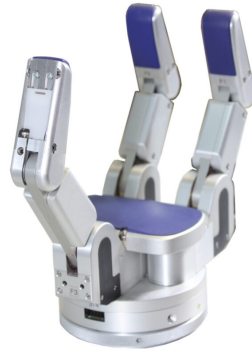
FIGURE 2.8. Image of a Barrett Hand (Barrett Technology, 1990–).
