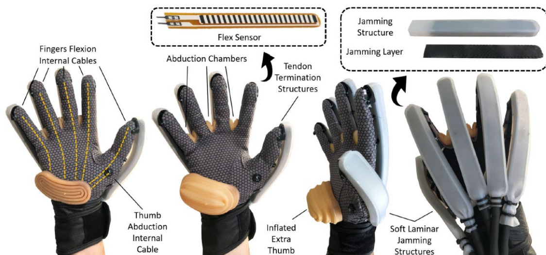
Figure 24 - The soft glove system of the device consists of a glove, a tendon-driven system, and a pneumatic system that is composed of four soft actuators and five laminar jamming structures. Five plastic tendon termination structures are stitched onto the fingertip regions of the glove. The tendon-driven system has a tendon connected to each of the tendon termination structures and an extra tendon that is connected to the thumb's interphalangeal joint region, facilitating the execution of the opposition motion. The soft structures are used for three different purposes: to perform abduction and adduction of the fingers, to enhance grasp stability by incorporating an extra thumb structure, and to modify the bending profile of the fingers. Three of the pneumatic chambers are connected to the region between the fingers, allowing for the execution of the abduction and adduction motion of the fingers. Another soft actuator was designed to function as a
