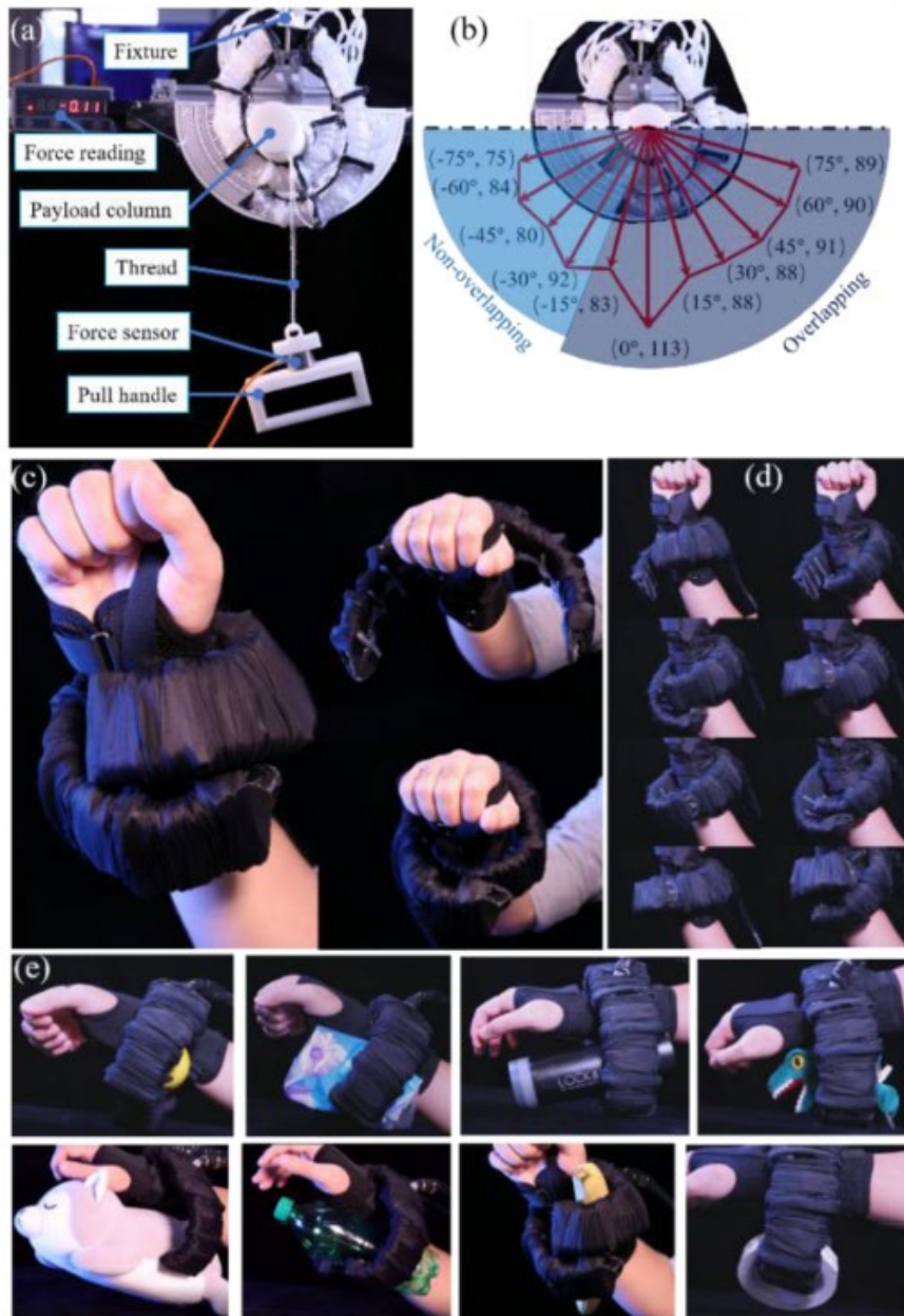
Figure 35 - Tests on the SRS flippers. (a) Test setup for measuring the maximum payload capacity of the bare-bone prototype at different orientation, (b) the payload plot indicating the SSR flippers were able to carry load as 50 times heavy as its self-weight; (c) when worn on human forearm, the flippers can open, close and compactly wrap around the arm, (d) the flipper were able to perform a combination of abduction/adduction manoeuvres in a folded state, displaying the advantages of the dexterity, (e) the adaptiveness to daily objects were demonstrated, a new hugging function was introduced, taken from Liu et al. 620
