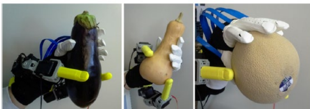
Figure 14 - Oddly shaped objects held by one hand, as demonstrated using the SR fingers, were taken from Wu et al. 504
