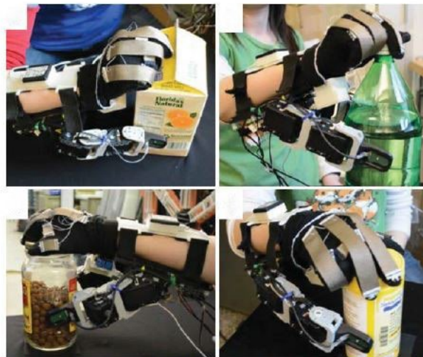
Figure 39 - Experimental validation shows a limited generosity to the user. Twisting off a bottle cap with the assistance of wearable robotic fingers was successfully tested on various types of bottles, taken from Wu et al. 732
