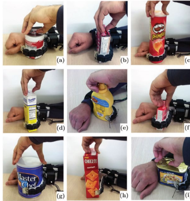
Figure 49- The soft sixth finger devised by Hussain et al., which tested its various grasp capabilities, was taken from Hussain et al. 1075 The soft sixth finger grasping various objects with different shapes and sizes: (a) tomato can, (b) chocolate pudding box, (c) chips can, (d) sugar box (e) mustard container, (f) gelatin box (g) coffee can (h) biscuit box (i) meat can. The device is intrinsically-compliant and adopts itself to the shape of the grasped object.
