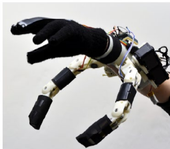
Figure 16 -The new SR Finger Prototype contains 4 DOF, including servo-actuated abduction and cable-driven flexion, taken from Wu et al. 514
