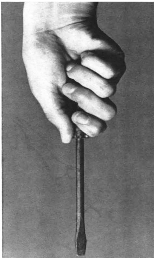
POWER GRIP is one of two basic working postures of human hand. Used when strength is needed, it involves holding object between flexed fingers and palm while the thumb applies counterpressure.
