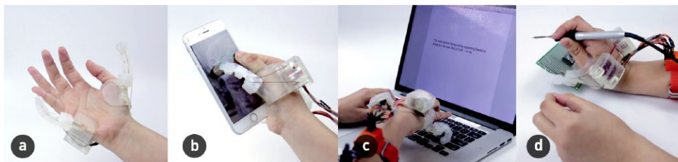
Figure 52 - The different grips of the Soft Robotic Fingers tested performing various tasks taken from Hu et al. 1078 a) The configuration of the system. b) performing multi-touch gesture with the soft robotic finger. c) the soft robotic finger supports keyboard typing. d) the fingers can hold and adjust the position of an object in tri-manual tasks.
