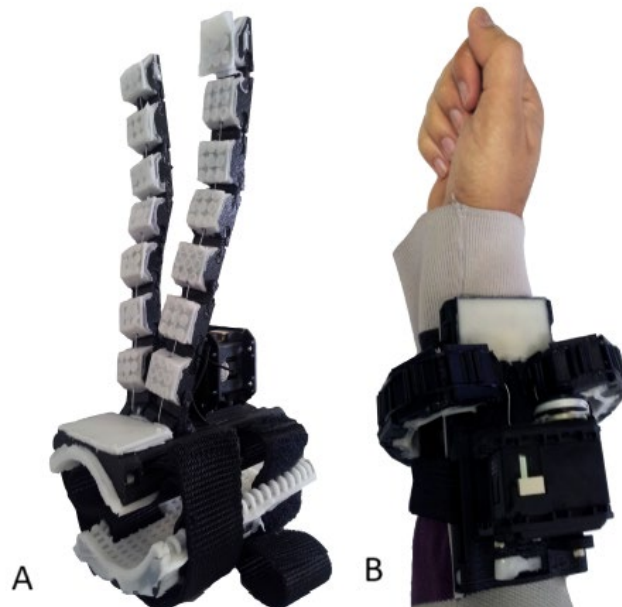
Figure 28 - (A) Final prototype of double soft sixth finger. (B) The double soft sixth finger in the bracelet position. Taken from Hussain et al.
