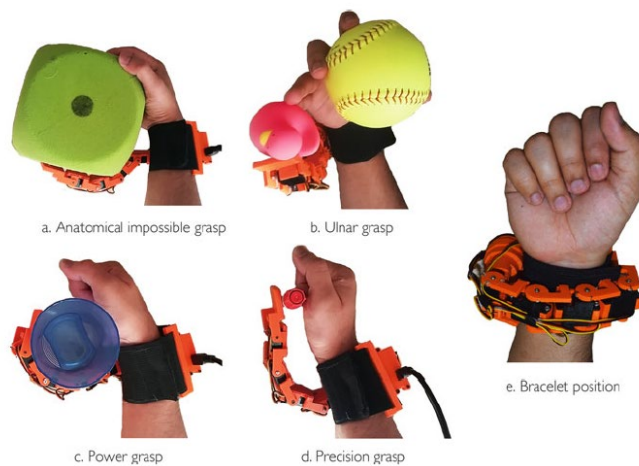
Figure 53 - The various important types of grasps as defined by Hussain and Prattichizzo using the same standard objects taken from Hussain and Prattichizzo 1079 . Examples of possible achievable grasps at working positions (a–d) and bracelet at rest position (e). In a and b, the robotic finger coordinates with the healthy hand to realise the anatomically impossible and ulnar grasp, respectively. While in c and d it interacts with the paretic hand to realise power and precision grasp
