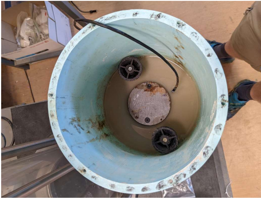
Figure 2-7: Displaced water from compaction past S_{r(opt)} captured by syringe
