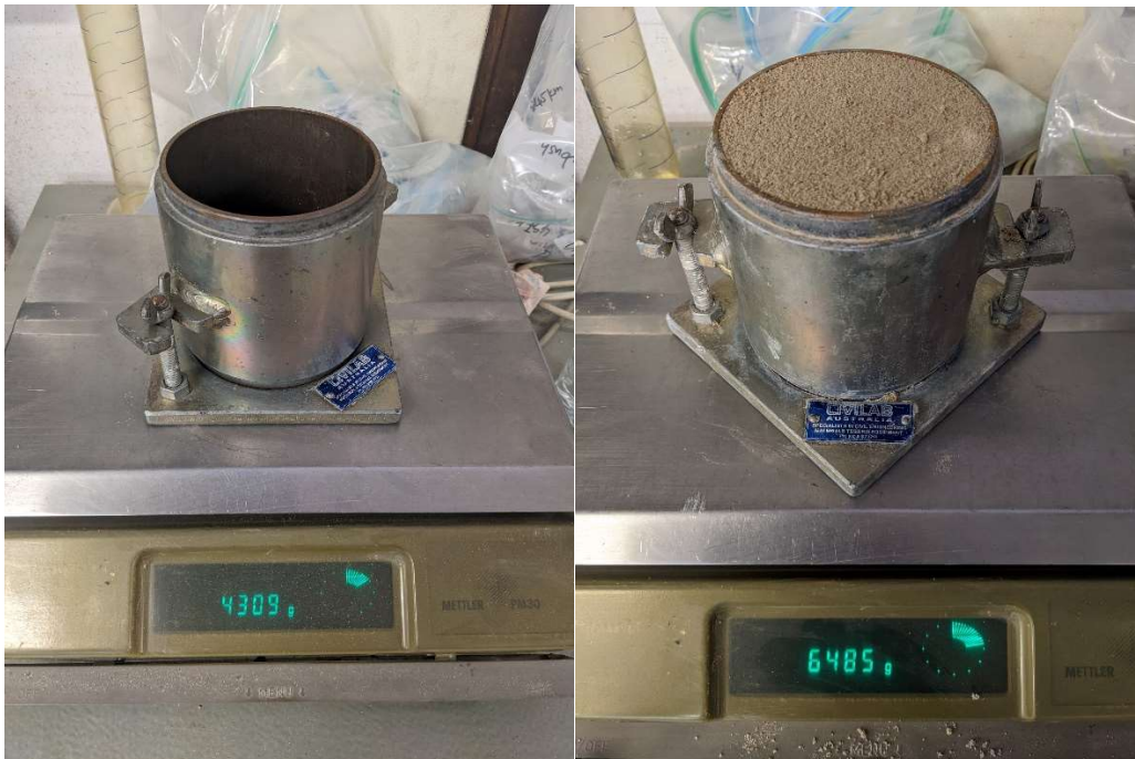
Figure A-4: Standard compaction testing of WCX silty sand sample
