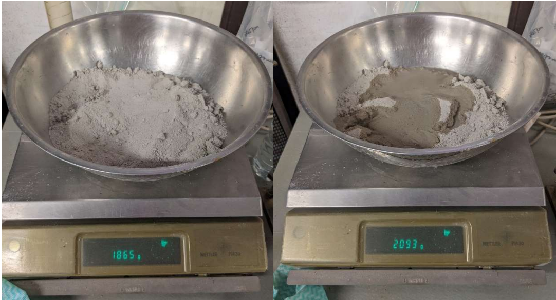
Figure A-3: Moisture conditioning of 2mm passing WCX sand samples
