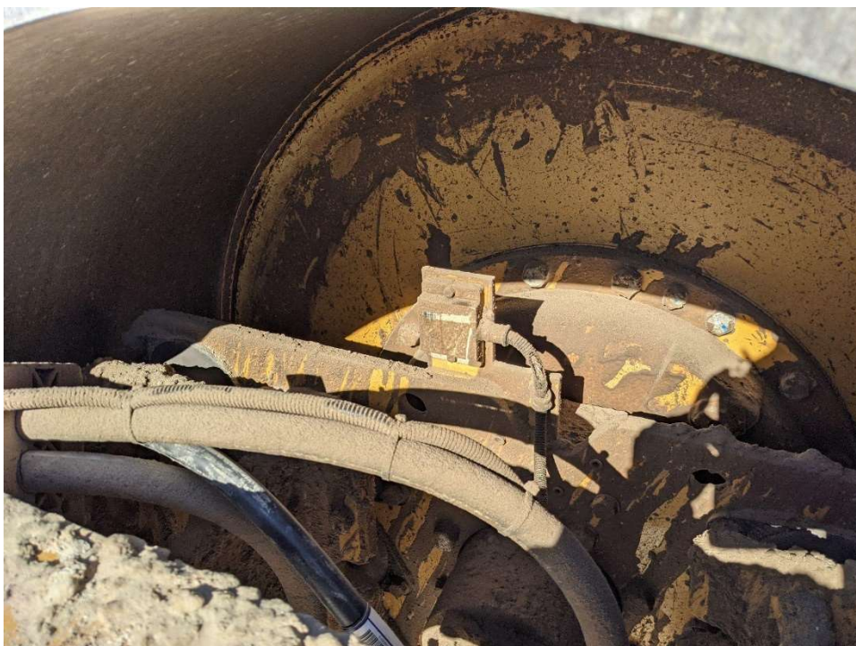
Figure 4-3: Accelerometer unit fixed to drum of a roller (20/4/21)
