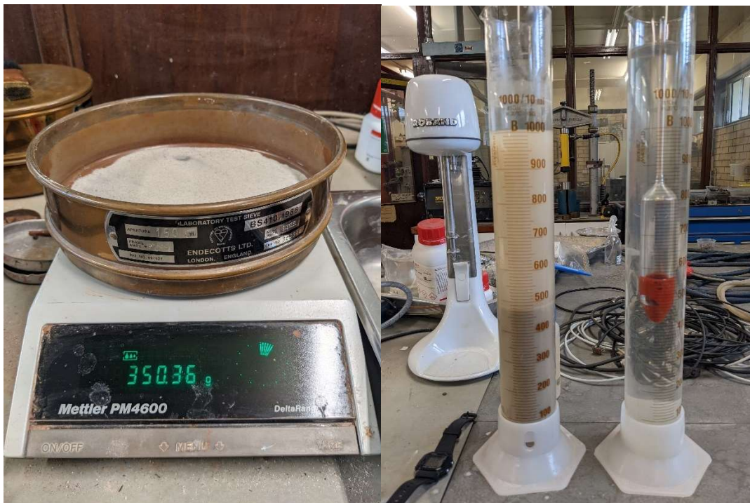
Figure A-1: WCX 2mm passing sample, PSD by wet sieve and hydrometer
